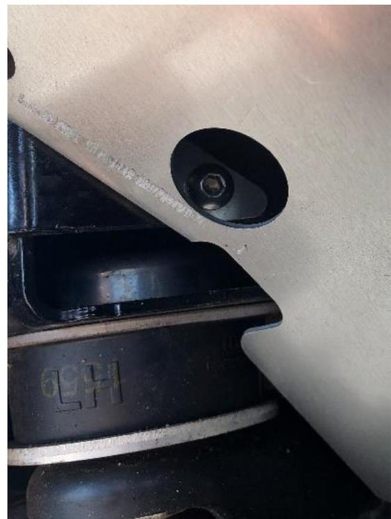
17. Using the rearmost hole in inner fender, loosely install EVO MFG inner fender liner onto the Jeep using a #10 bolt and nut. (Pictured)
