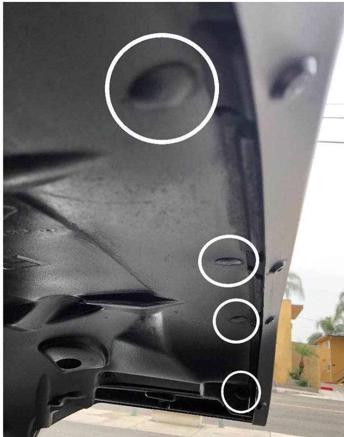
8. Remove the 2 button clips on the bottom rear of the factory inner fender liner.
