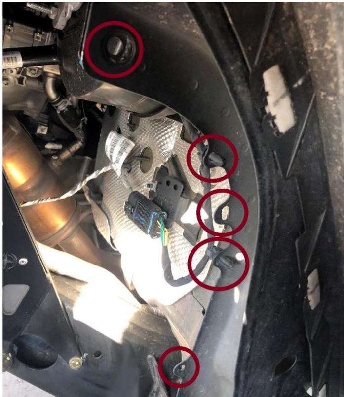
14. On driver side slip one of the supplied clip nuts onto top hole in pinch seam positioned as pictured.
