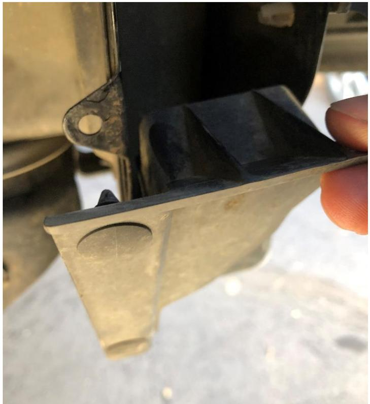
12. On the passenger side, remove the top plastic clip from pinch seam and plastic wire retainer using a clip removal tool.
