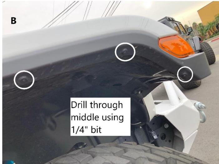
7. Using a plastic fastener clip removal tool remove the 4 button clips located just inside of the clips removed in the previous step.
