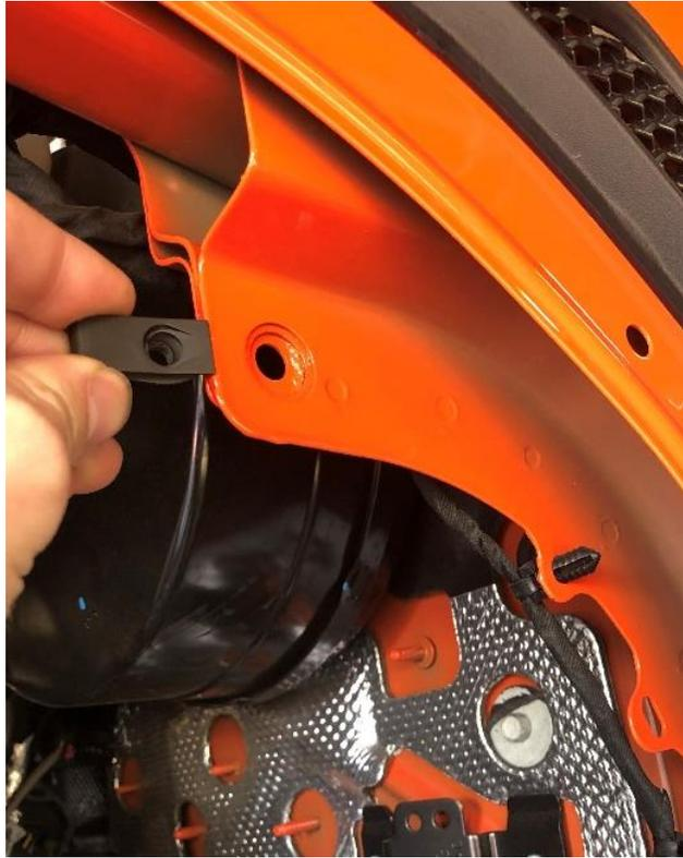
15. On passenger side pinch seam, insert clip nut over hole in the plastic wire retainer (behind the pinch seam), where push clip used to be. (pictured)
