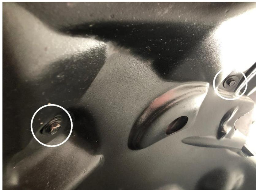
10. Remove button clip located at front body mount.
