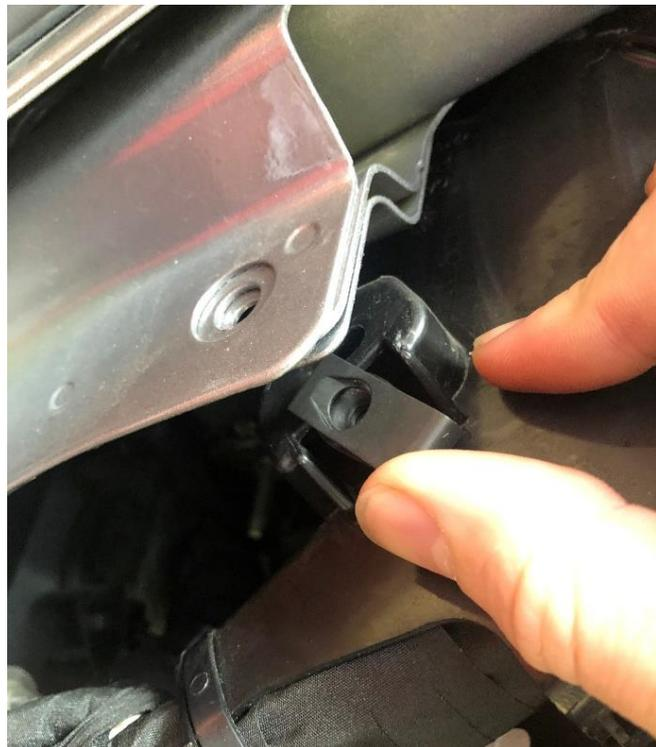
16. Using the forwardmost hole in inner fender, loosely install EVO MFG inner fender liner onto Jeep mounting location using a ¼-20 bolt and nut. (Pictured)
