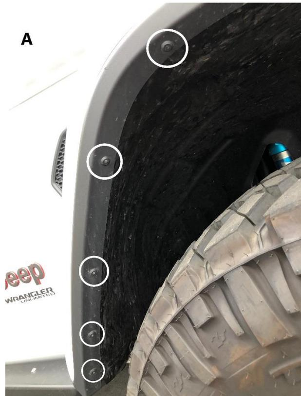
Once all 8 button clips have been drilled, remove all the clips completely.
