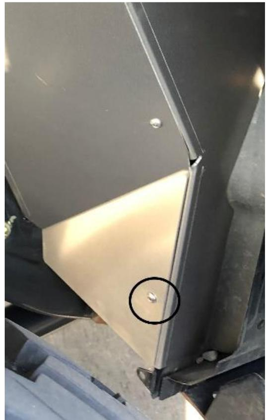
18. Insert a ¼"-20 bolt into hole in the rear panel. Once the bolt grabs onto the previously installed clip nut, tighten down to snug.
