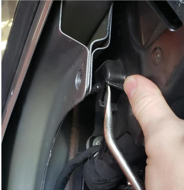
13. Remove wire fasteners from all locations referenced in picture on both driver and passenger sides.
