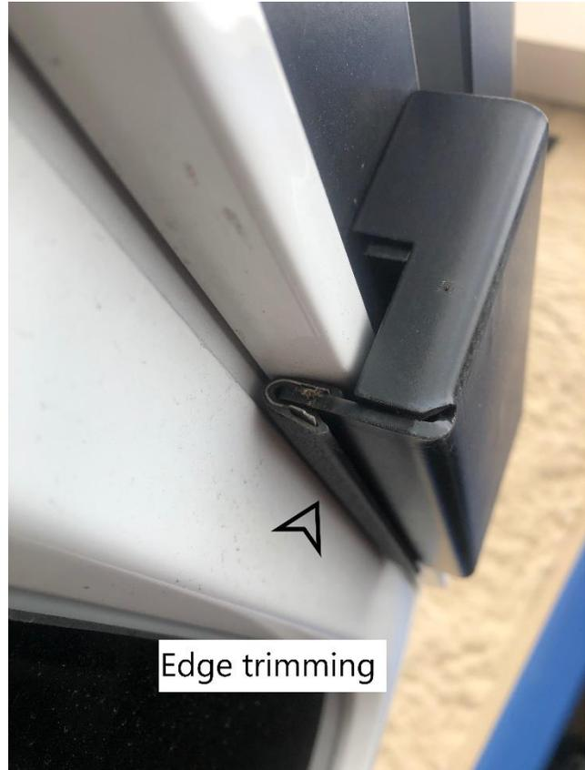
11. Insert bolt and washer from top down of upper mounting plate and thread into outer rail mount. Lower edge with trim should be grabbing underside of hardtop drip rail.
