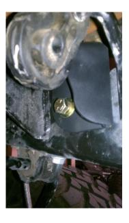
37. Install lower shock mounts to EVO Rockstars using supplied larger spacers, one on each side of shock. Do not use small spacers that may be attached to the lower end of the shocks. Use supplied M12 bolt.
