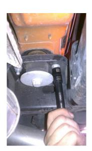
10. On passenger side rear exhaust hanger at frame. Bend hanger upwards about ¾" with pry bar.
