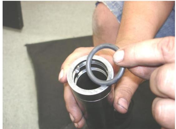
30. Make sure felt seals are fully pressed into grooves on both side of seals. Pack all seals with grease.
