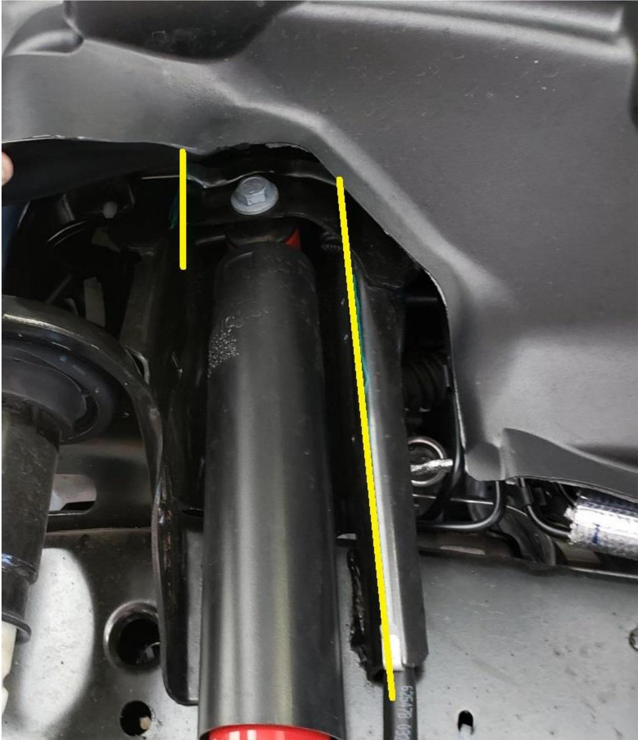
Removed section, Driver side inside of bracket shown:
