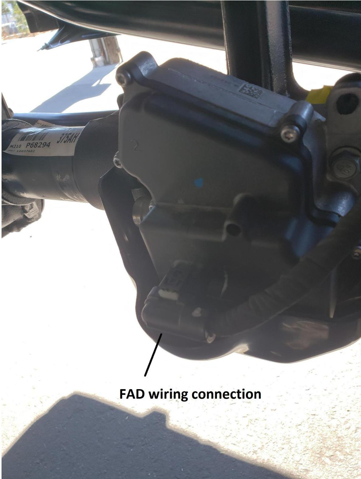
7. Rubicon Models: At differential, carefully pull outward on red clip at axle differential until clip stops. It should move out about a 1/8". Then depress clip button and disconnect clip/connection.
