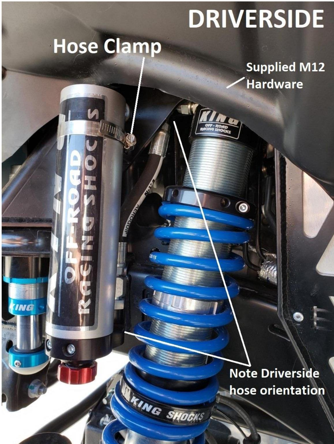
24. Using supplied hose clamp and previously installed reservoir mount. Wrap clamp around reservoir body and through slots in mounting bracket. Insert end of hose clamp into screw end. Turn screw on hose clamp to tighten reservoir to tower.
