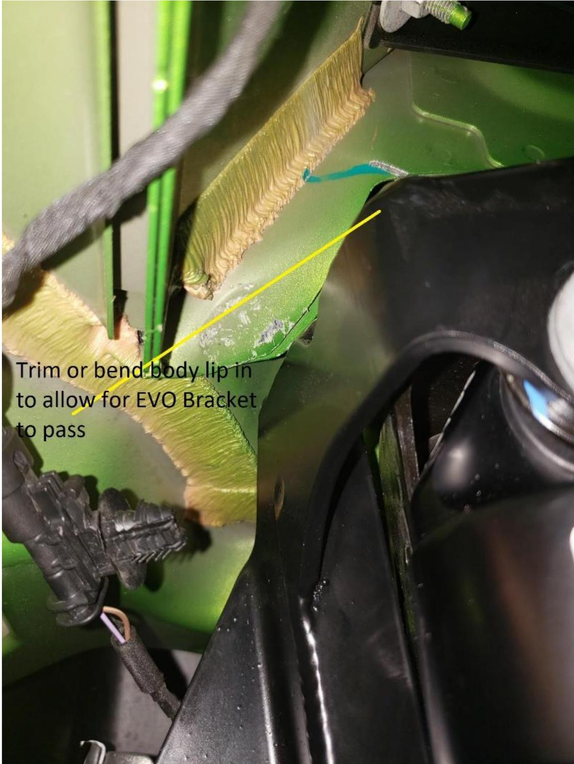
20. Insert rear coilover support tower over factory rear shock mount at frame.
