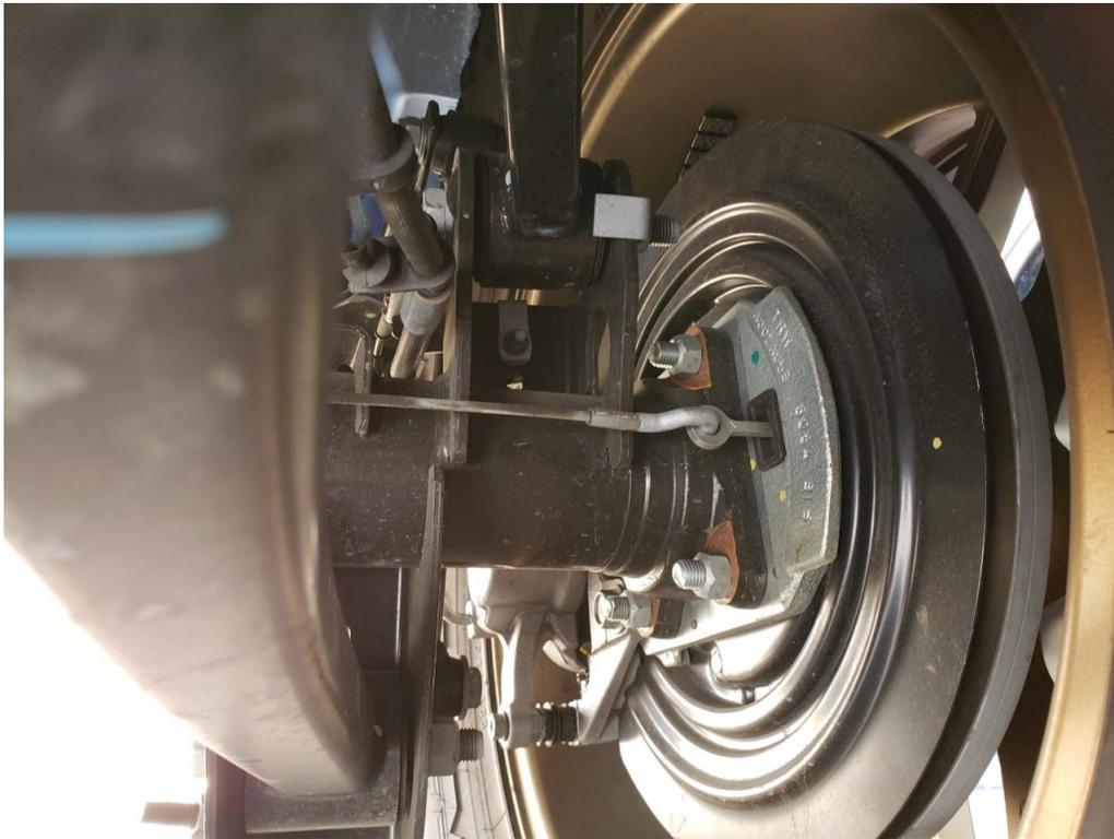
15. Install EVO rear brake line bracket to axle as shown with supplied hardware.
