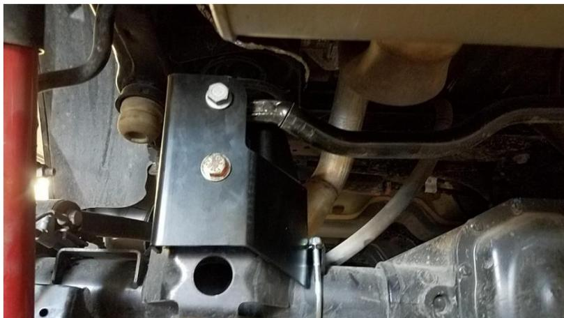
19. At rear upper shock mount at passenger frame. Using a cutting tool (if removing) or a chisel/hammer: cut off or bend in rear section of pinch seam as shown giving clearance for bracket to pass. Use touch up paint if needed.
