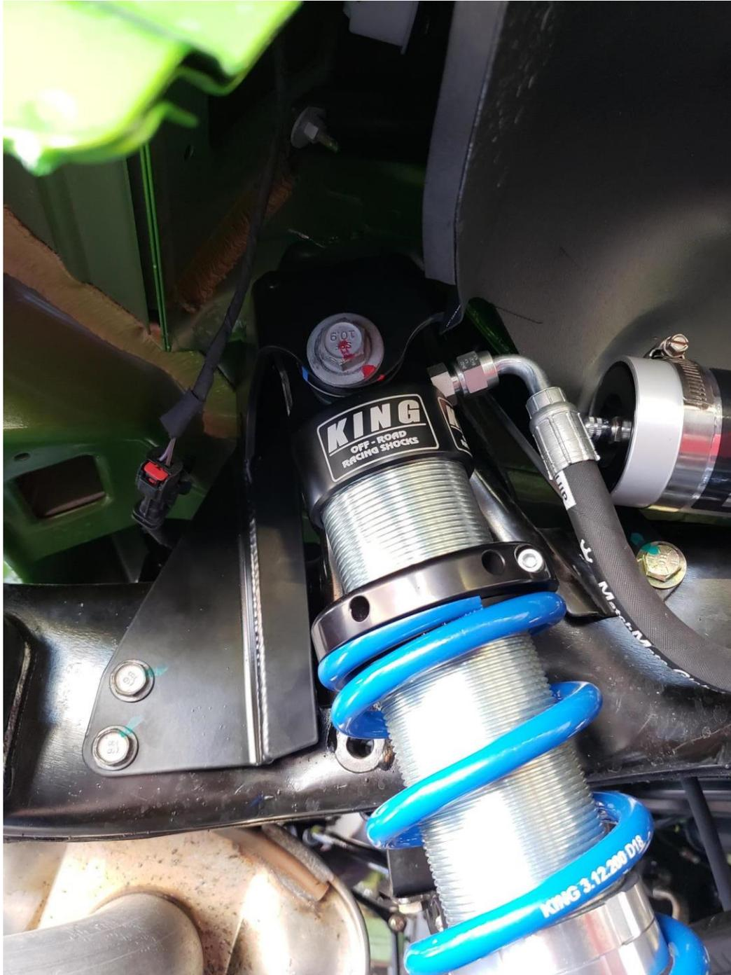
29. Install lower shock into axle mount/EVO Shock skid with factory bolts.
