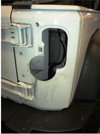
10. With all nutserts installed, install RockSkin to fender with supplied ¼-20 Stainless flat head screws
