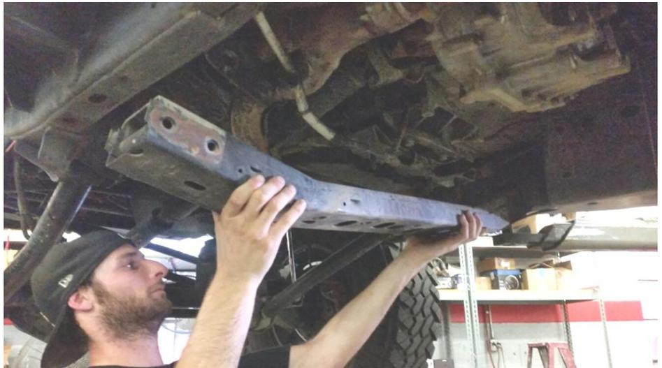
7. Insert the EVO HD transmission crossmember into place on the vehicle, sliding the passenger side up and in position along the factory frame rail.
