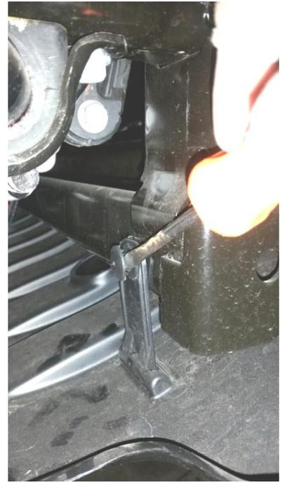
2. Remove factory bumper top fascia section that sits between the grill and bumper and is held in place by two plastic grommets which are slotted for a screwdriver. Unscrew the two grommets and pop off the top section fascia. If you are having troubles unscrewing the two grommets you can place a flathead screwdriver between the screw of the grommet and the grommet pry the grommet screw loose. Once the screw is removed the grommet will easily lift from the frame.
