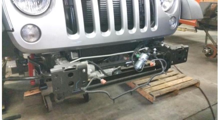
7. Carefully remove the factory bumper from the vehicle.
