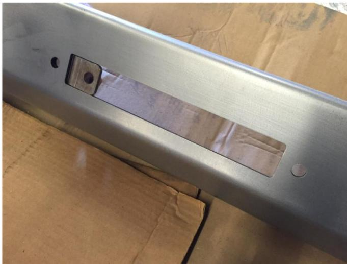
Install EVO Fairlead Jog Plate on driver side for Centered Winches
