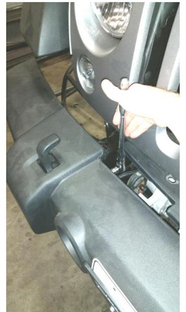
4. (2012 and up Jeep JK's) Remove the two bolts that hold the factory vacuum pump.
