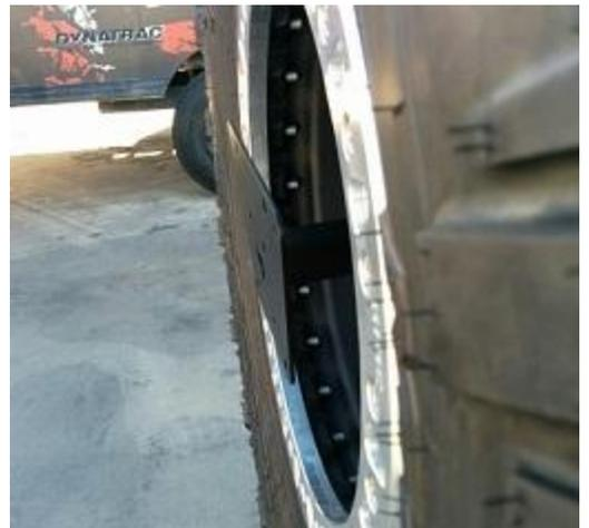
5. Use the hardware supplied by RotoPax to attach their bracket to the EVO MFG Mounting Plate. (The RotoPax universal mount is shown)
