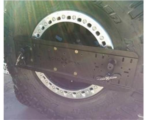
6. The mounting hardware or gas can needs to be pulled tight against the tire to apply tension and keep the gas can from rattling. You will need to use a 9/16 wrench (a ratcheting wrench works well for this) to tighten the bolt until it does. This bolt can be accessed from the underside without removing the RotoPax hardware.
