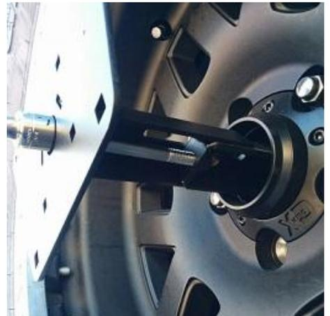
4. Use a 9/16 socket with extension to tighten the Mounting Plate until it is flush with the tire.
