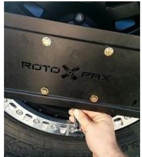
7. To install for use as a license plate relocate and not a gas can mount, thread the supplied  $\frac{3}{4}$ " long bolt locknut and washers through the slot in the center. Slide the bracket to the desired depth and tighten the bolt, clamping the sliders together.
