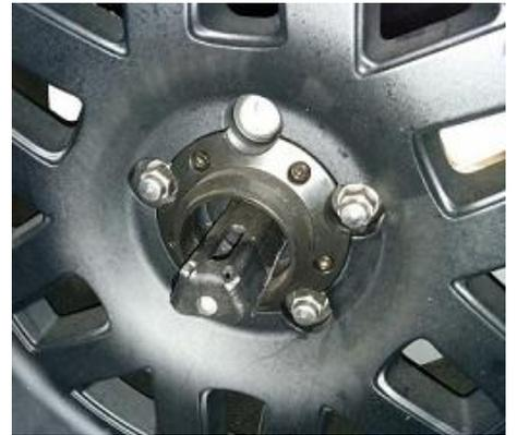
3. Slide the Mounting Plate over the Stud Plate and thread the 4" long bolt through and into the nut in the stud plate
