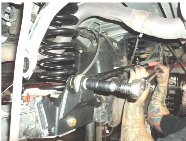
40. Install springs into lower axle mount, smaller end of spring should be mounted on the axle side. Larger end of spring goes up while retaining the factory rubber coil spring isolator
