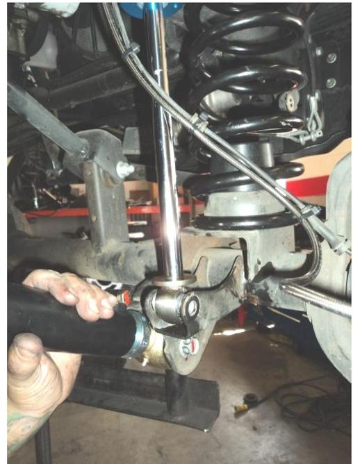
13. On both driver and passenger side, drill and 5/16" hole in the center of the spring mount on axle.
