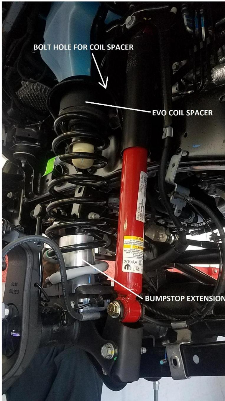
15. Insert supplied  $\frac{3}{8}$  x 2" bolt into front bumpstop extension. Place bumpstop with bolt inside (bore side up) factory spring and reinstall factory coil spring and rubber isolator on top of coil into its original location on both the frame and axle. Isolator will now be seated on the EVO coil spacer. Axle may need to be lowered to install.
