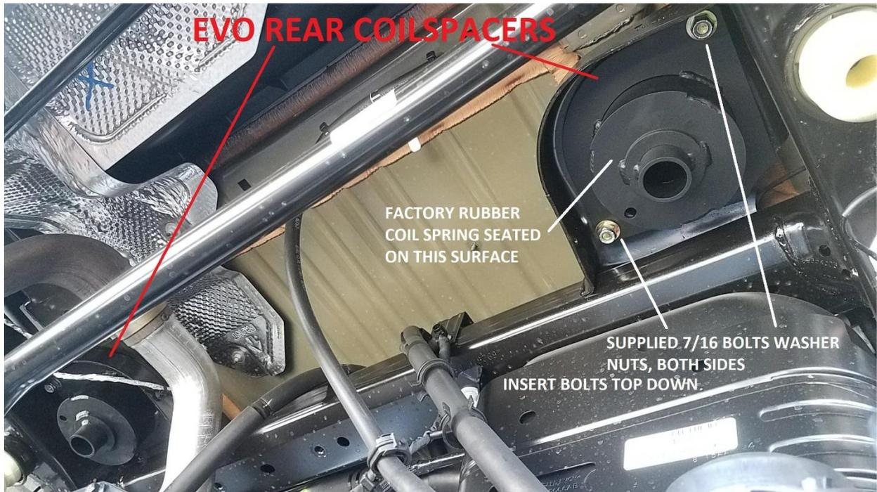
38. Reinstall driver and passenger side coil springs into place keeping factory rubber isolator on top of spring. Be sure to align nub on isolator so that it inserts into hole in EVO brackets. The spring isolator will now be resting on the EVO coil spring spacer.
