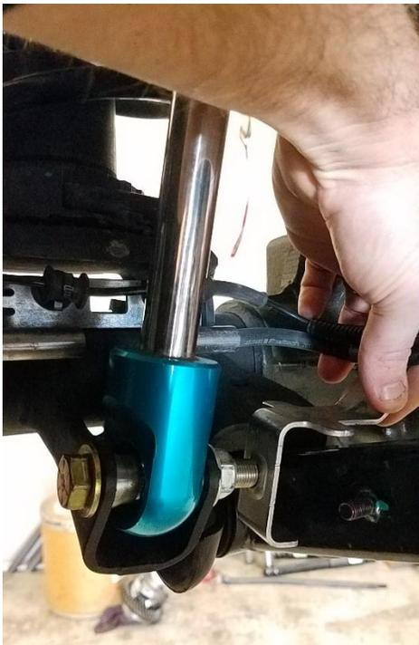
that once attached to factory lower arm to ½” and install on shock bolt after shock bolts have been torqued. Use M12 nut supplied with EVO Enforcer Control Arms. Series: Shock nut, brake line bracket, Flange Nut.
