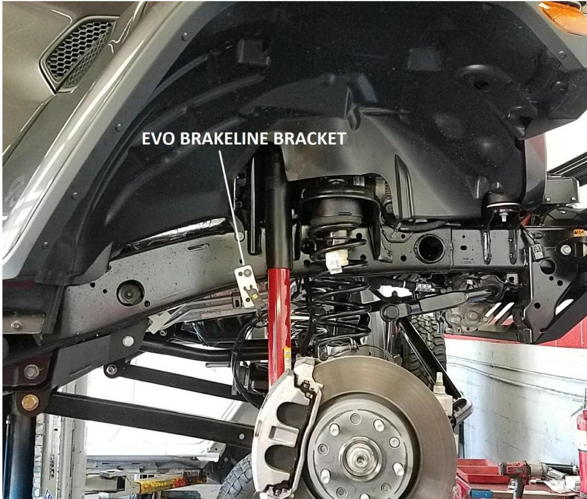
18. Install factory brake line to the new lower location on the EVO brake line extension bracket. **Be very careful moving line into new location. The factory hardline will need to be slightly manipulated to be relocated. Do not use tools or pinch/crack the line.**
