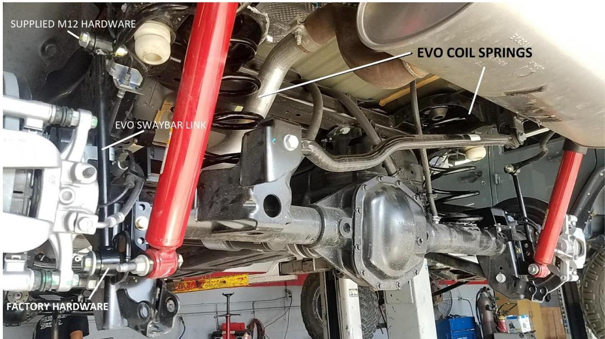
36. Assemble supplied rear swaybar links. Using light oil such as WD 40. Lubricate inner surface of link loops. Tap or vice in supplied rubber bushings. Lubricate inner surface of rubber bushings. Tap or vice in supplied swaybar tube sleeves.
