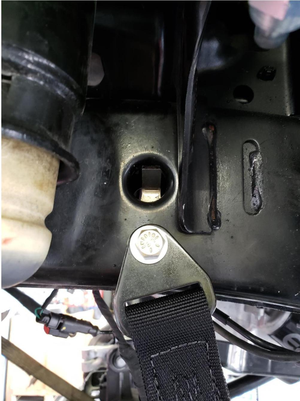
4. On axle side. Using supplied 1/2" bolt, washer and nut install lower end of limit strap loop to the inner factory JL shock mount tab.
