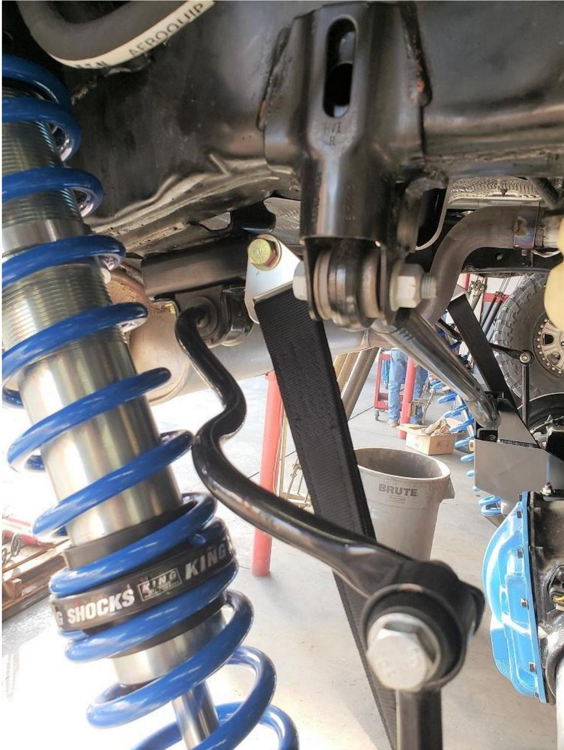
7. On rear axle. Drill/enlarge existing hole in rear lower control arm brackets to  $\frac{1}{2}$ ". Using supplied  $\frac{1}{2}$ " bolt, washers, nut, install lower rear limit strap loop end to drilled hole in axle bracket. Use additional washer between axle bracket and limit strap loop to space limit strap off bracket. Nut can be accessed from underside of bracket by tapping nut to wrench end and inserting upwards.
