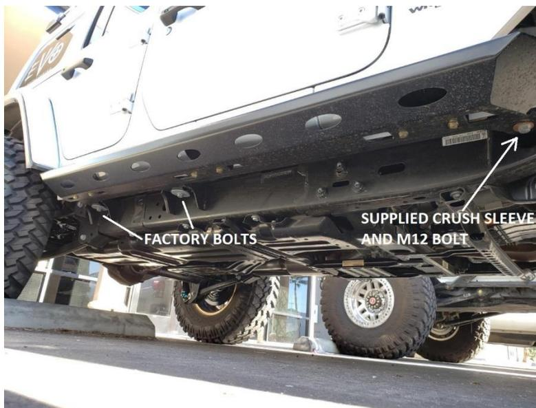
10. Using a jack, apply an upward and inward pressure to the bomber rail, lifting it up to an approximate level/as installed location.
