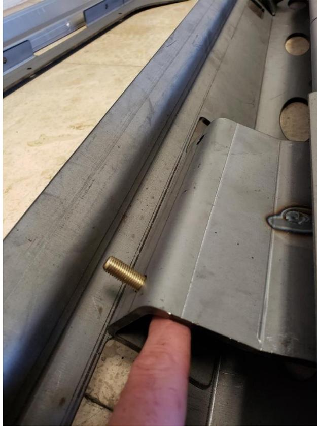
7. Using supplied 5/16" hardware, loosely install the remaining 4 5/16" bolts, washer and nuts at the inner seam mounts.
