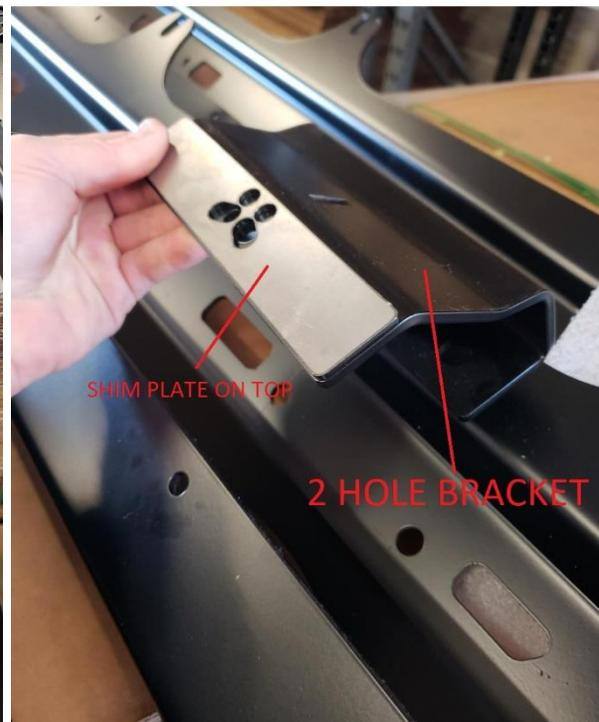
5. From the top down install all 10 button head screws. Keep the 3 bolts at the inner seam mounts loose, just before tight. All other 7 can be tightened at this time.
