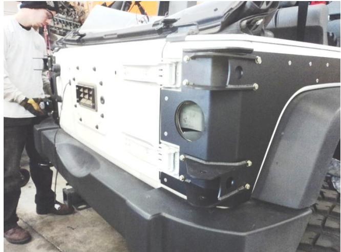
6. Once all 4 brackets line up the armor hole carrier level to body with alignment bolt installed and mark all 15 holes to be drilled on the mounting plates.
