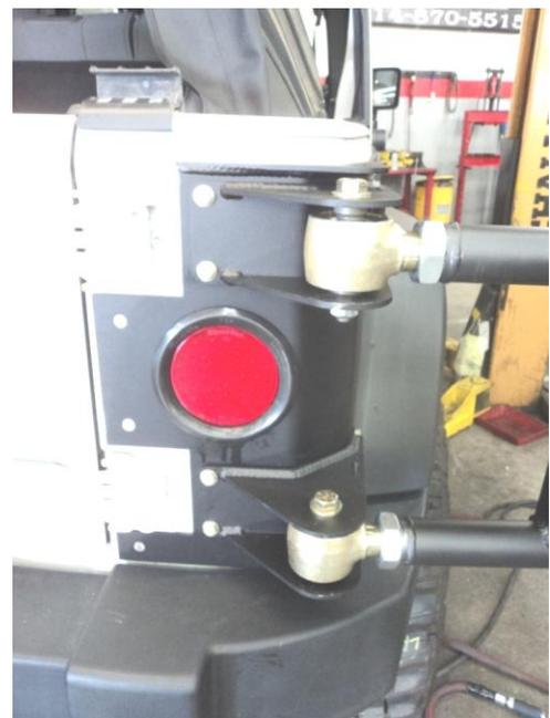
14. Install wheel mounting plate to spare tire/wheel with the plate on the back side wheel, just as would be installed on the vehicle. Stud on plate should be sticking out towards front side wheel.
