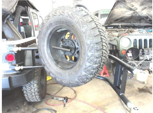
17. Slide T handle through the center hole of the wheel mounting plate and tread into tire carrier. Tighten. You do not need to over tighten this connection. Make sure tire is fully seated against tire carrier and T handle is snug and secure.
