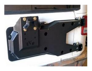
11. Using 6 of the 8 bolts that were surrounding the vent in the center of the tailgate (removed in step 5), thread them into the remaining 6 openings in the Tailgate Tire Carrier. These can be accessed using a 13mm socket and extension as shown.
