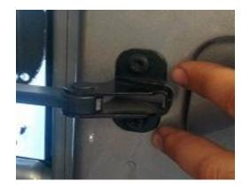
5. Remove the 8 bolts around the vent in the center of the tailgate as well as the plastic trim covering the hinges. Set the bolts aside to reuse later
