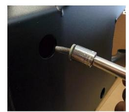
12. Once all the bolts are threaded to the tailgate, fully tighten all bolts to tailgate only.
