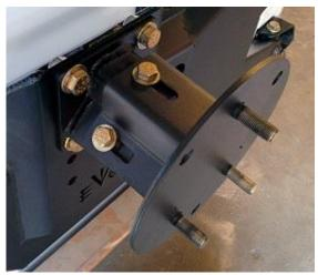
17. Install your wheel and tire and fully tighten
