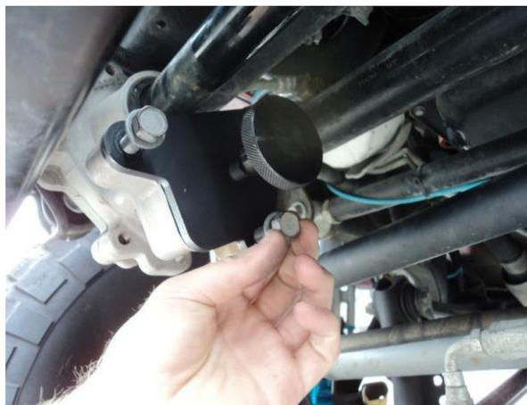
5. Install the EVO NoLimits Rubi Swaybar Disconnect as shown using factory hardware
