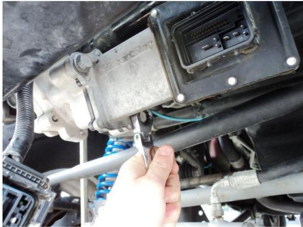
3. Remove factory swaybar actuator. With a screwdriver push into circular chamber and verify the actuator movement.
