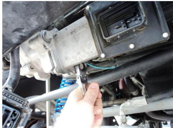
3. Remove factory swaybar actuator.
