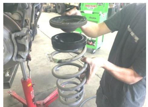
25. Slowly and carefully raise axle with jack until lower shock mounts line up with axle mounting bolt holes. Make sure upper coil springs and isolators are properly centered in coil spring perches on top and bottom
