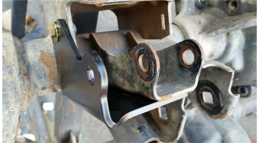
5. **Loosely** install the EVO MFG Front shock relocation bracket (**DO NOT TIGHTEN at this point**). 2 Bolts on the underside of the factory shock mount with 3/8" hardware and side bolt with 5/16" hardware.
