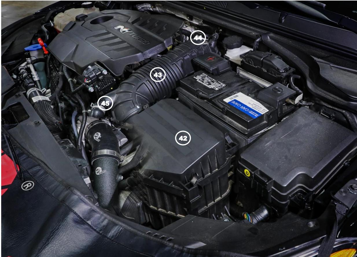
55. Reinstall the air intake box into the vehicle (42)
