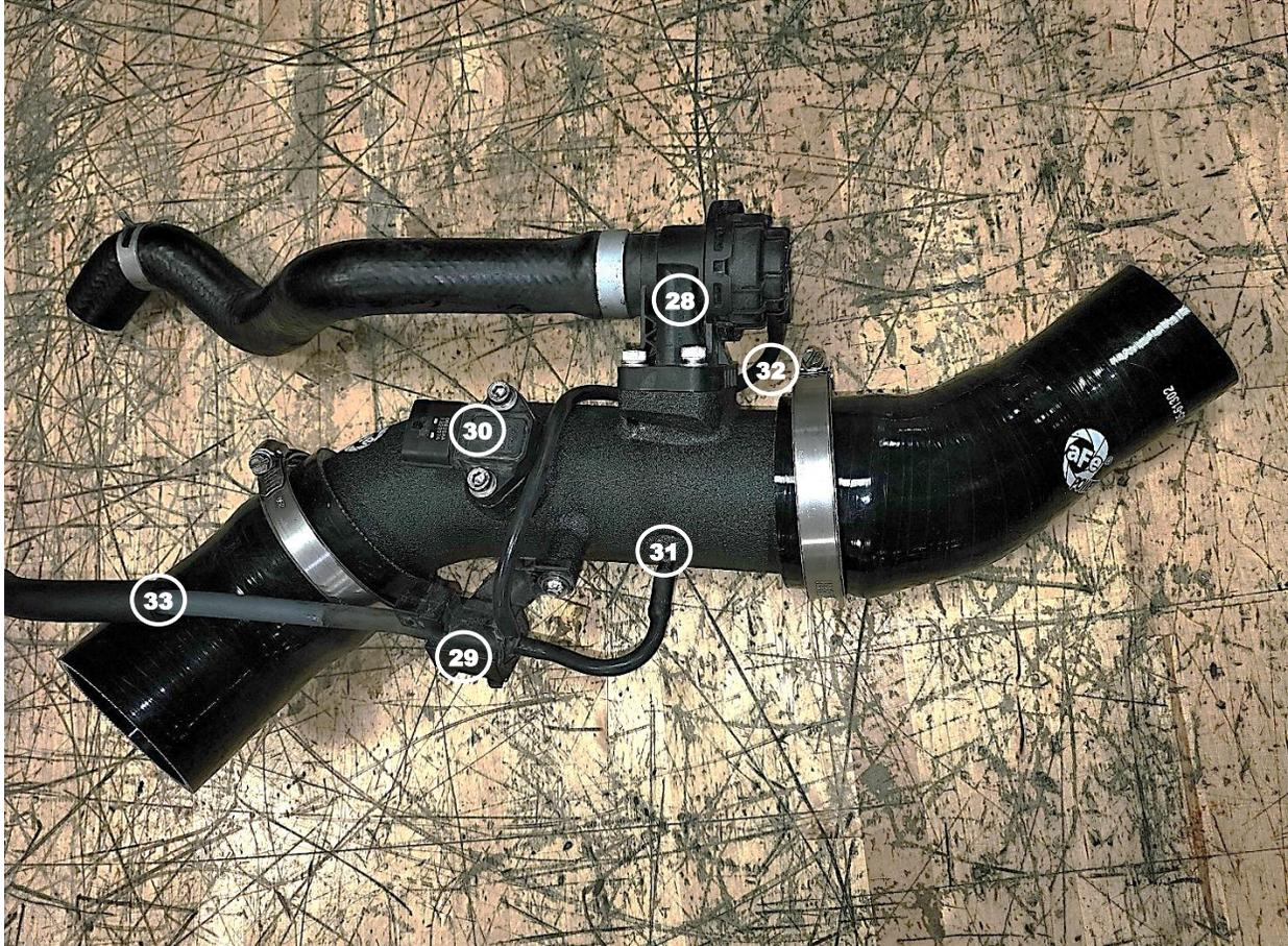
37. Transfer the factory diverter valve onto the aFe cold side charge pipe (28). Secure it with four (4) of the supplied M6 x 1 x 20mm screws and M6 washers.
