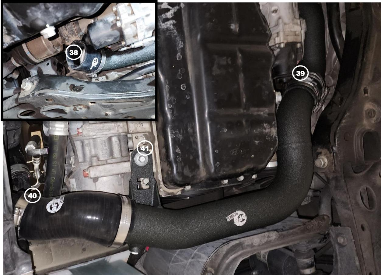
**Note: Be sure to thoroughly clean all oil residue off of the connections before installing any of the aFe charge pipes into the vehicle**
