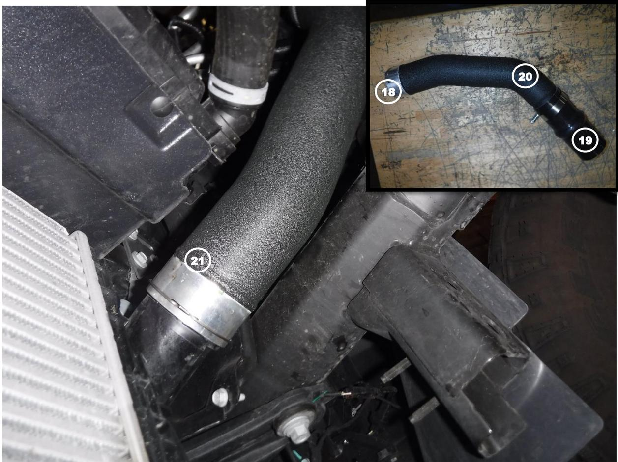
**Note: Be sure to lubricate the O-ring with grease to prevent it from tearing during installation.**
