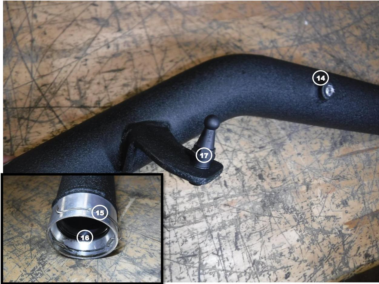
**Note: Be sure to use thread sealant on the plug or sensor to prevent any leaking**
