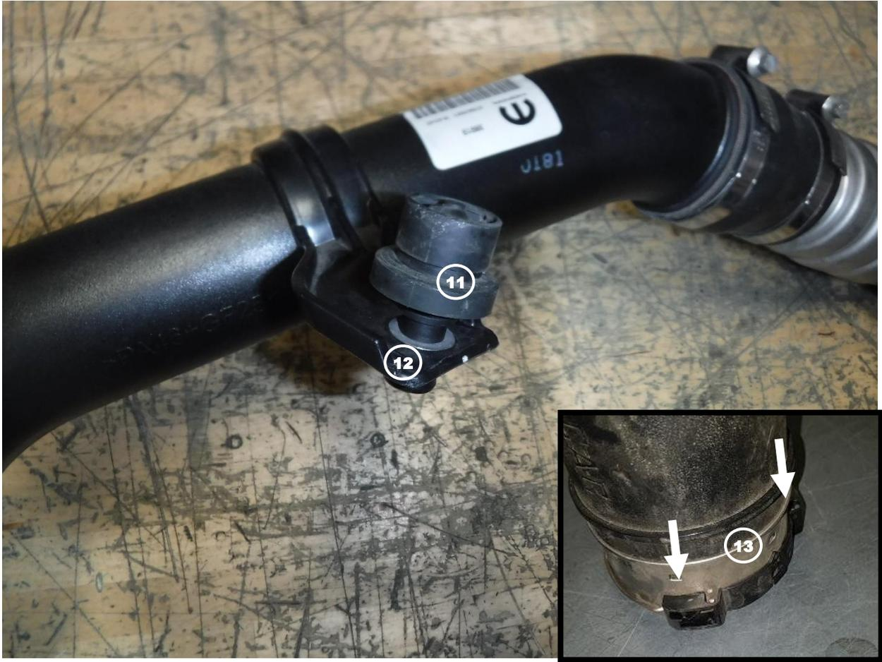
15. Remove the air intake grommet from the mounting pin (11) if it is still connected and set it aside to be installed later.
