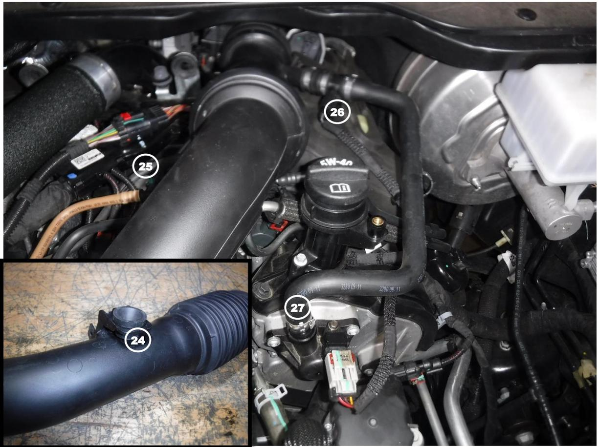
30. Install the factory air intake tube mounting grommet into the intake tube (24)
