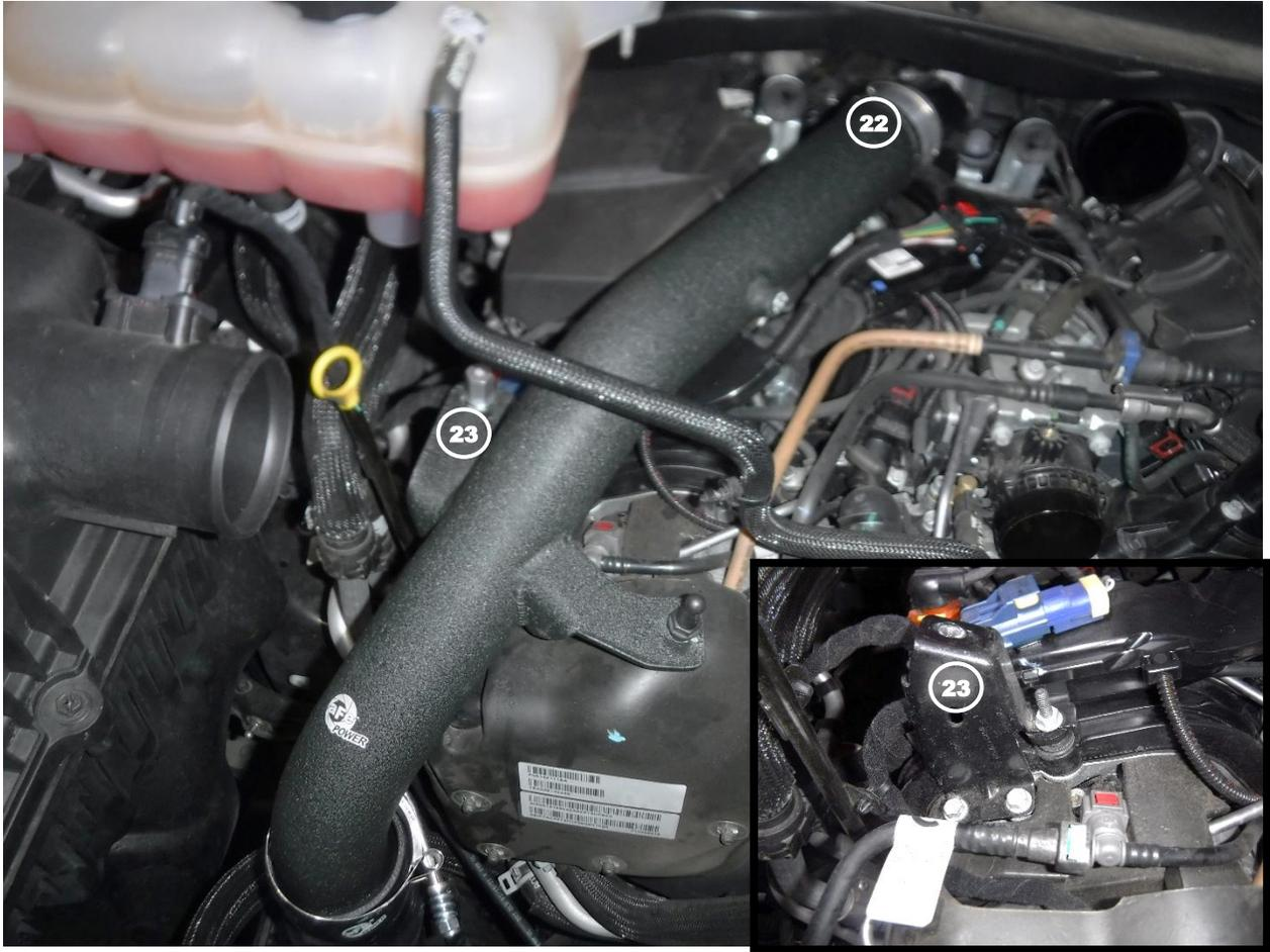
26. Install the upper aFe hot side charge pipe with one 3.00" t-bolt clamp into the vehicle, first connect it to the coupling from step 24, then connect it to the turbo outlet (22)
