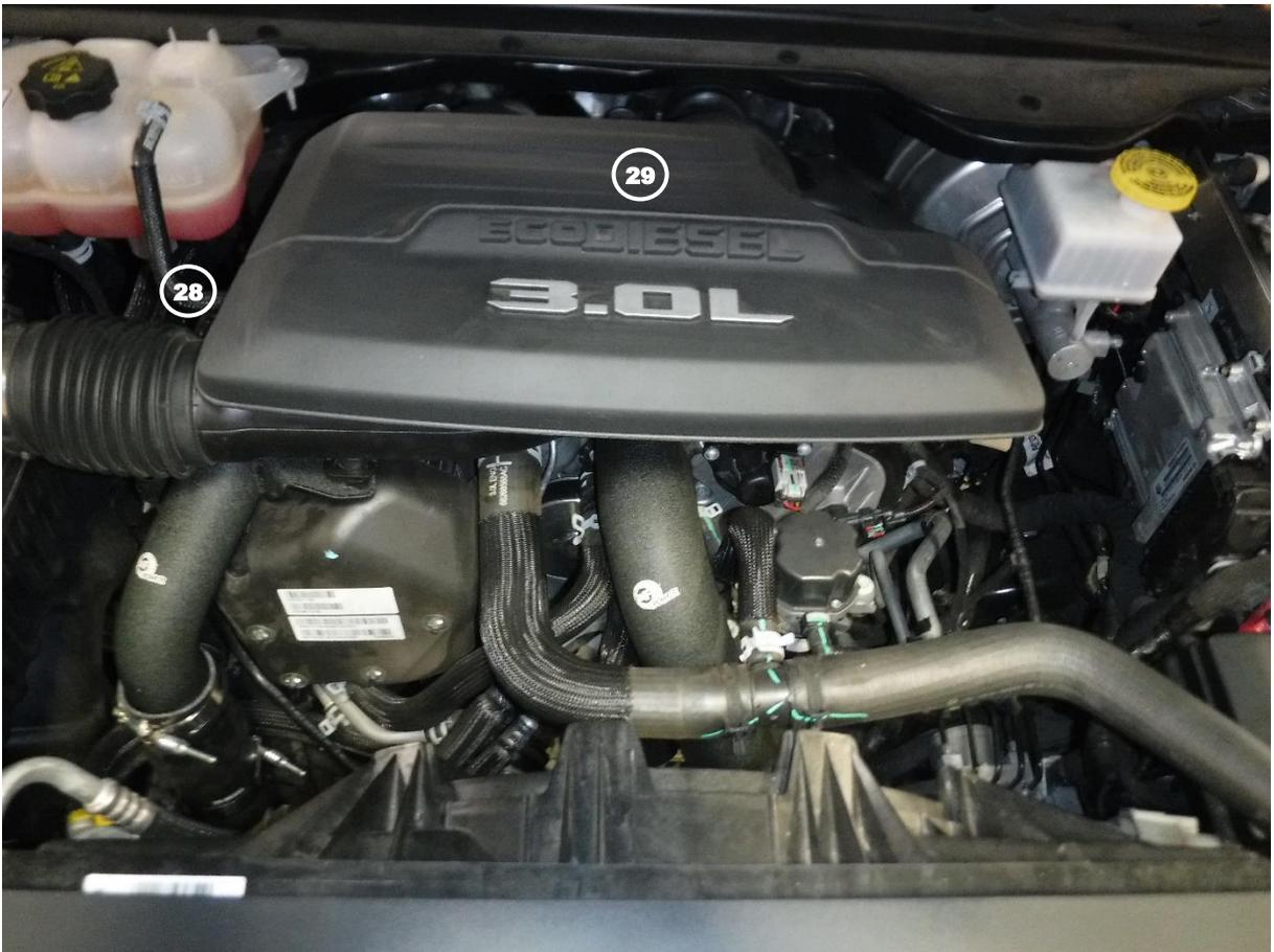
35. Reconnect the coolant overflow hose to the intake tube (28).
