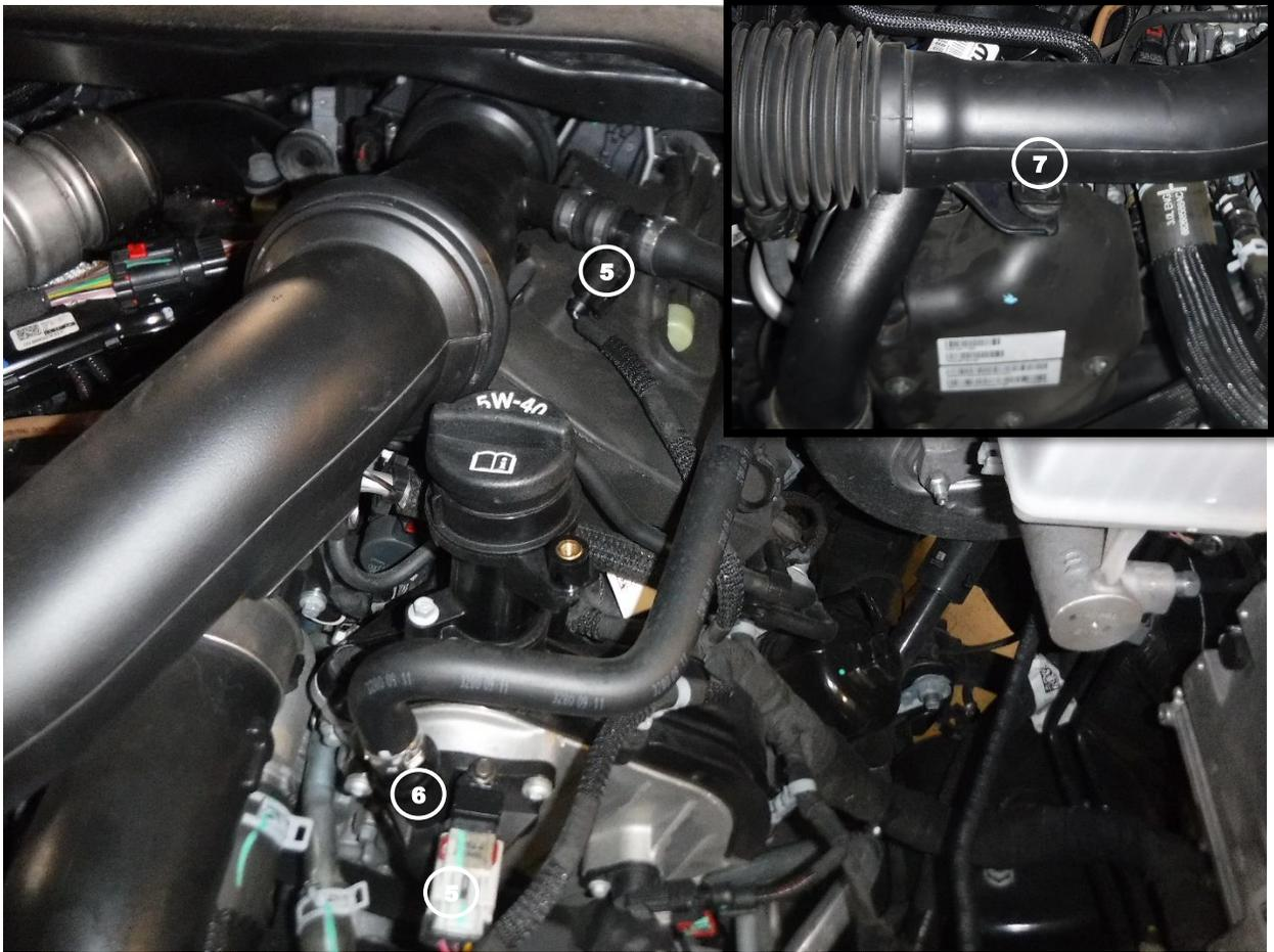
7. Disconnect the Positive Crankcase Ventilation (PCV) wire harness (5) from the air intake tube.
