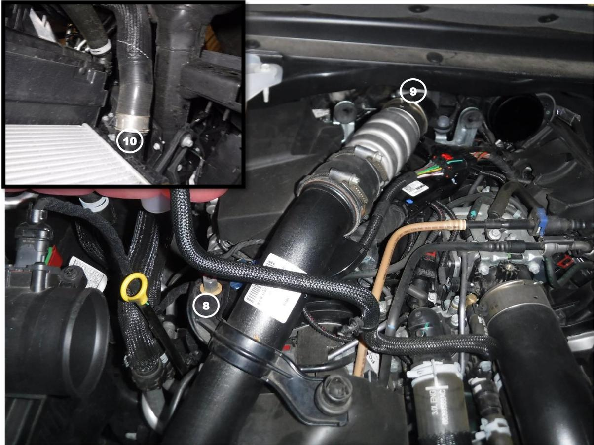
11. Remove the screw securing the hot side charge pipe to the engine ⑧
