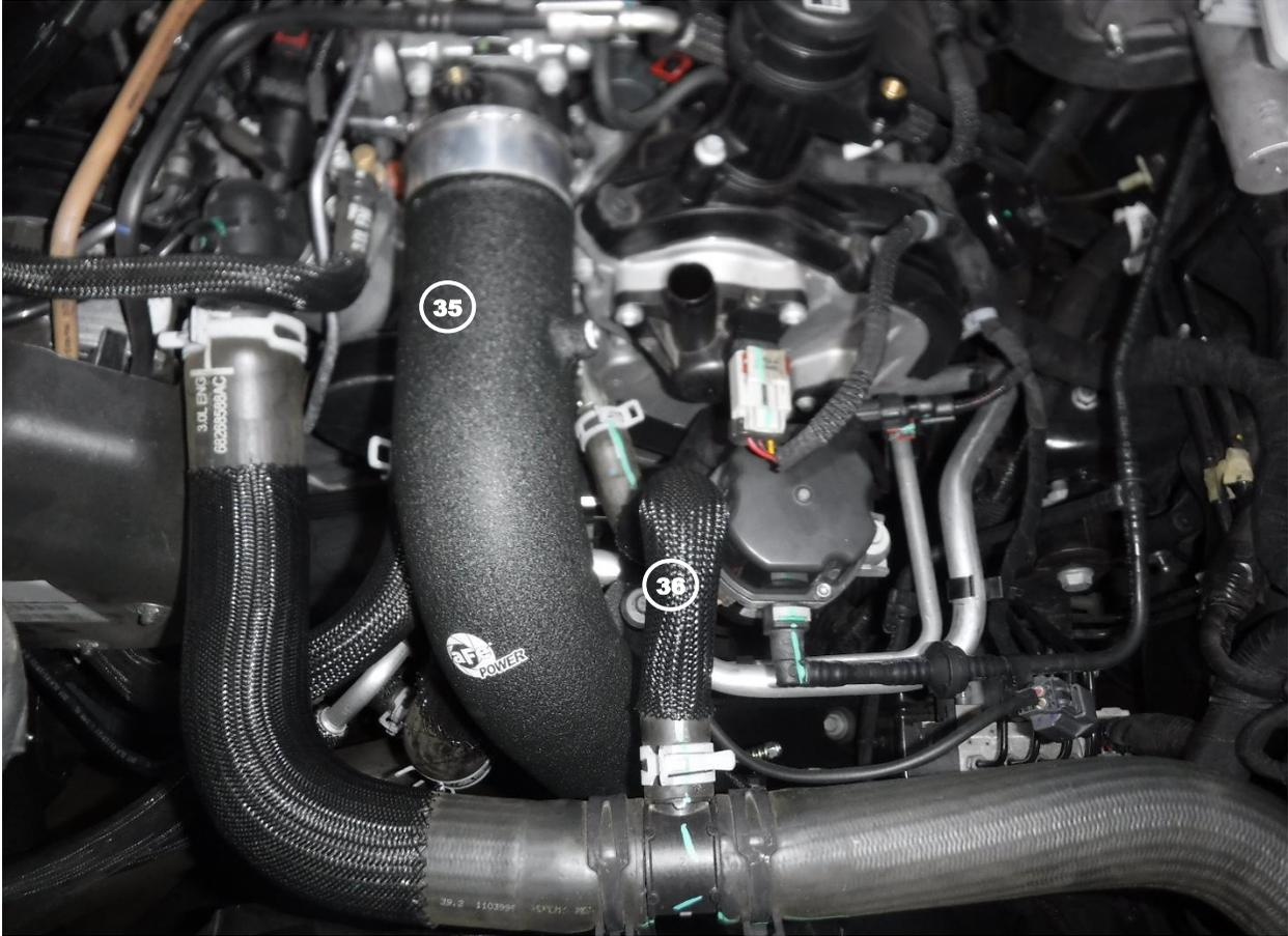
40. Install the upper aFe cold side charge pipe with one 3.25" t-bolt clamp into the vehicle, first connect it to the coupling from step 38, then connect it to the engine inlet (35).
