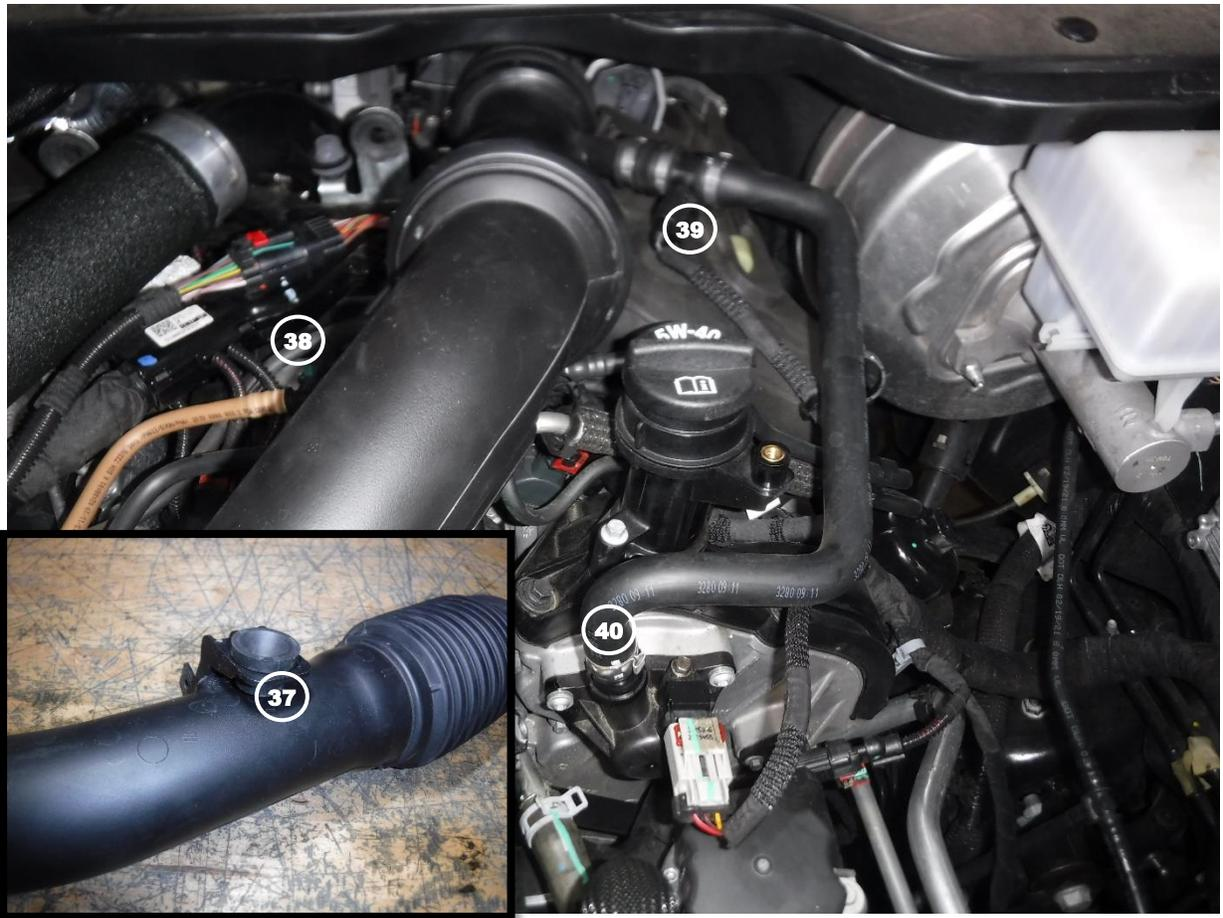
44. Install the factory air intake tube mounting grommet into the intake tube (37)
