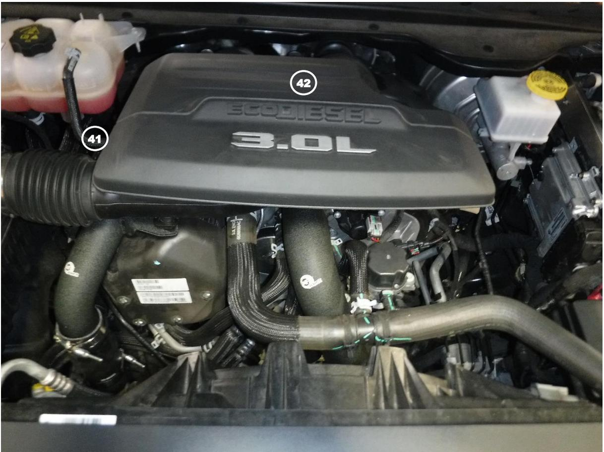
49. Reconnect coolant overflow hose to the intake tube (41)
