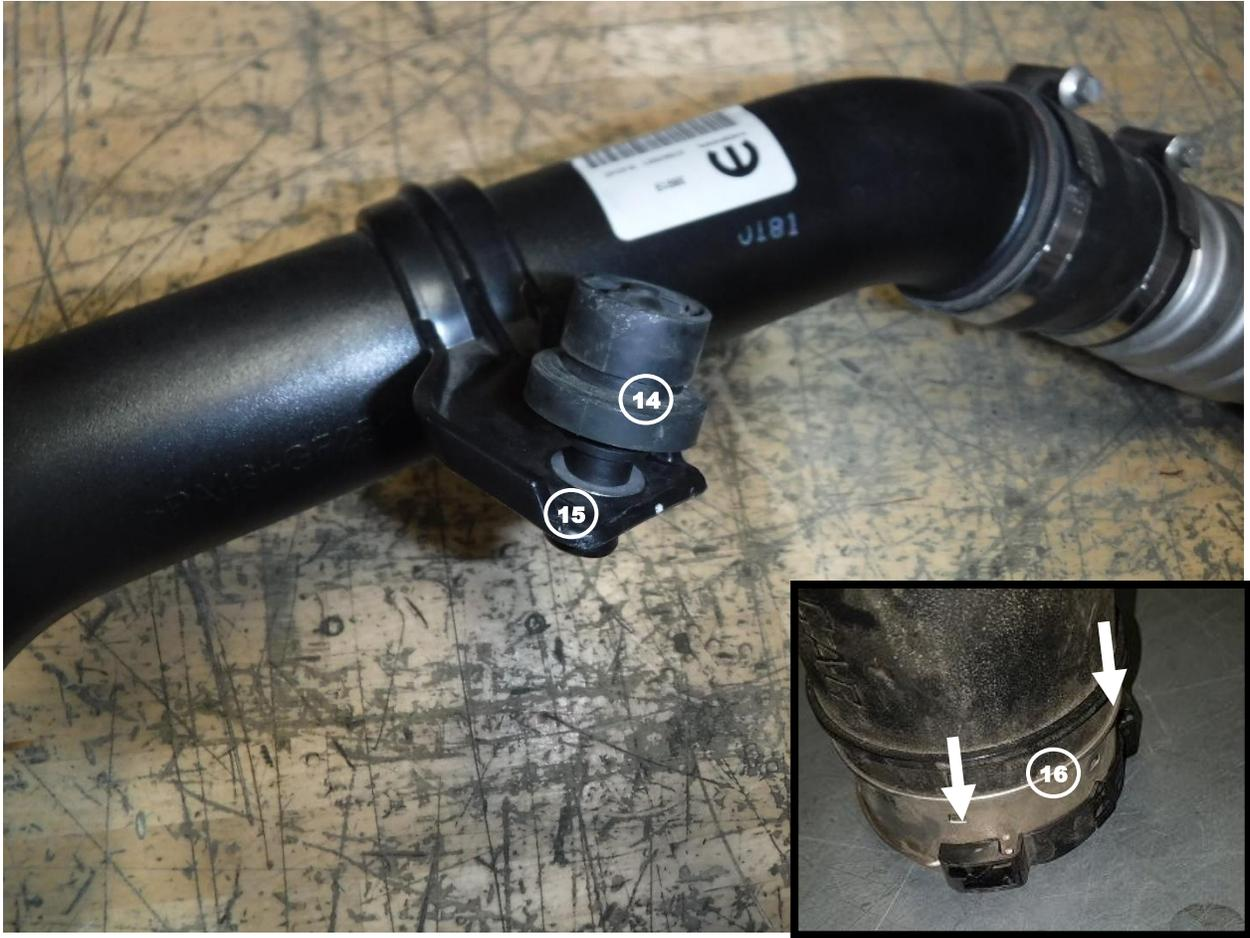
19. Remove the air intake grommet from the mounting pin (14) if it is still connected and set it aside to be installed later.
