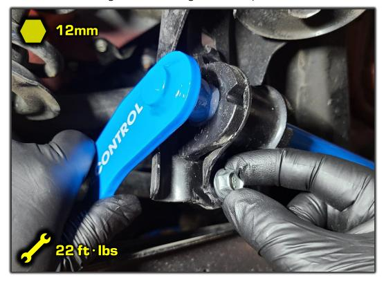
8R Match the length to the factory end links. Position the heim joints to be perpendicular to each other and tighten the jam nut.
