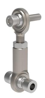
9R Install the end links onto the lower control arms. In some cases, the end link may feel like it is a bit tight to go into the lower control arm. If this happens, loosen the lower shock bolt a few turns to let the control arm open up. Once the end link is installed, you can retighten the shock bolt and end link bolts.
