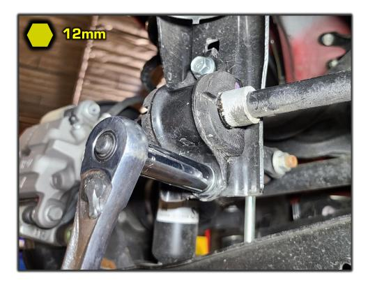
4R Remove the rear sway bar from the vehicle.
