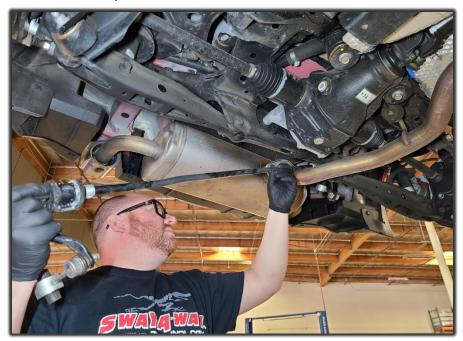
5R Lay out the factory sway bar with the aFe Control sway bar to match the orientation.
