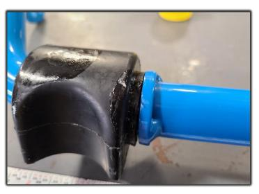
Install the factory bracket and hardware to secure the bar to the frame mounts. Tighten the nut and bolt evenly, however, make sure to fully tighten the nut <u>before</u> fully tightening the forward bolt.
