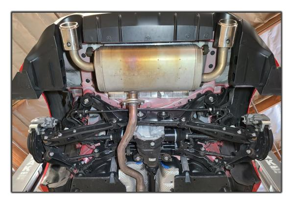
2R Unbolt the end link from the lower control arm. Repeat on other side.
