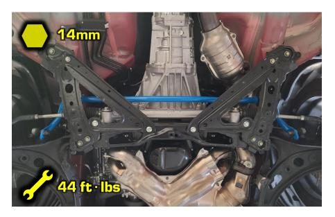
13F Install the end link onto the sway bar end. The hole closest to the end is the softest setting. The hole furthest from the end (shown) is the stiffest setting. Tip: Add some thread locking compound to the end link stud to ensure long lasting tightness.
