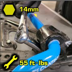
12F Reinstall the sway bar assembly back onto the vehicle in the same manner as removal.
