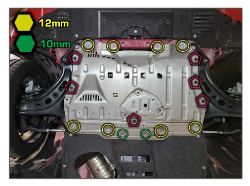
3F Remove the center felt undertray by unfastening the (9) bolts.
