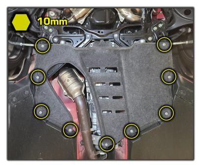
4F Remove the passenger side plastic under panel by unfastening the (3) bolts, and (10) pop clips.
