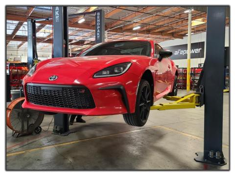
2F Remove the front aluminum undertray by unfastening the (8) bolts-12mm socket, (2) bolts-10mm socket, and (6) pop clips.
