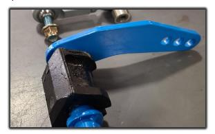
7R Install the aFe CONTROL sway bar in the same manner as factory removal.
