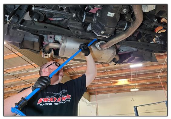
Reinstall the stock bushing brackets using the factory hardware.
