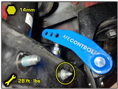
10R Install the bolt & Nylock nut onto the sway bar end as shown. The hole closest to the end is the softest setting. (Shown) The hole furthest from the end is the stiffest setting.
