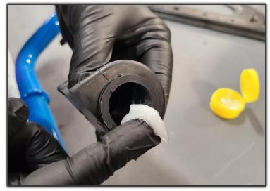
Make sure the ring stop is installed towards the sway bar centering ring.
