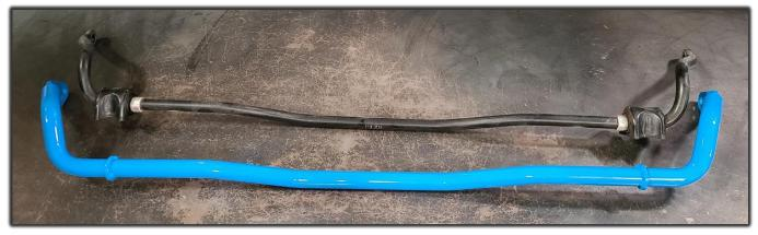
10F Lube the inside surface of the bushing using the provided grease. Spread open the bushing and install onto the sway bar.
