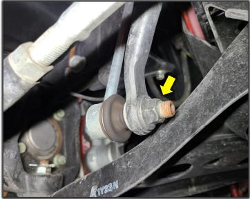
7F Unbolt the sway bar frame mounts (10) bolts.
