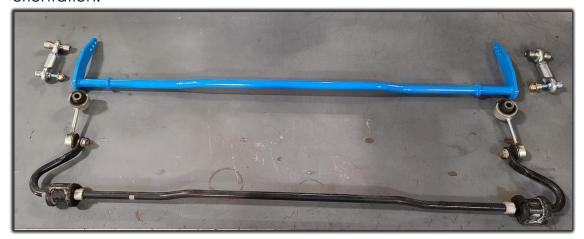
Lube the inside surface of the bushing using the provided grease. Spread open the bushing and install onto the sway bar.
