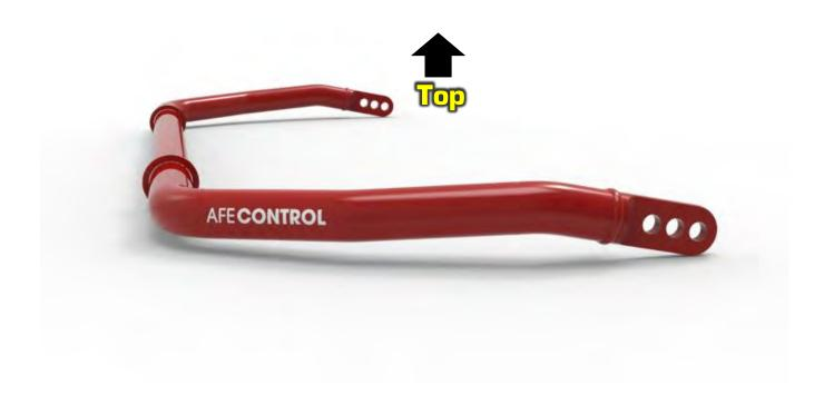
Install the aFe CONTROL sway bar in the same manner as factory removal. Follow the same movements as before but in reverse order. **Tip: It's a good idea to keep** the sway bar in the poly bag it ships in when inserting it into the car. This will avoid any unnecessary scratches to the bar. Once the bar is in place, remove the poly bag.
