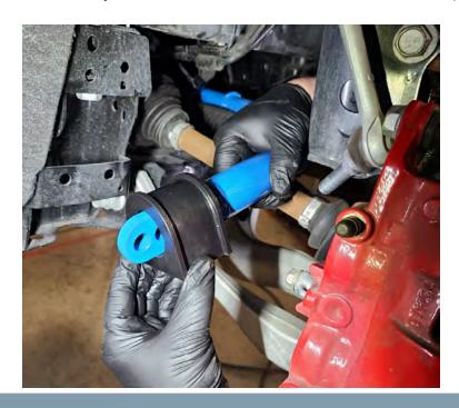
Before you get the bushing all the way to its final position, apply the included grease to the sway bar in the area before the centering ring. As you slide the bushing in, try to pry it open with your fingers. Once you get it into place rotate it a few revolutions to ensure the grease is evenly distributed.
