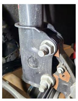
Unbolt the abs sensor from the upright using an 8mm socket.
