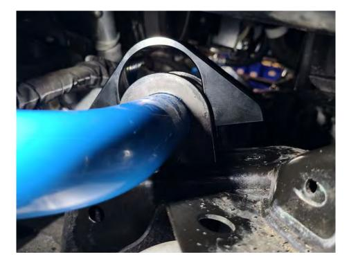
12F Install the end link onto the sway bar end. The hole closest to the end is the softest setting. The hole furthest from the end (shown) is the stiffest setting.
