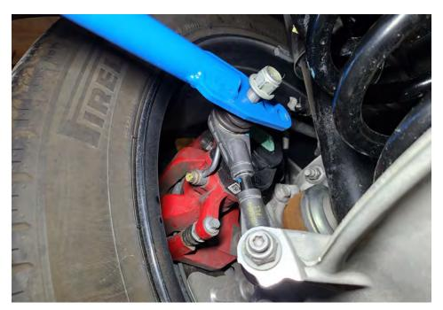
10R Reinstall the exhaust heat shields and rear wheels. You are now done with the rear sway bar installation.
