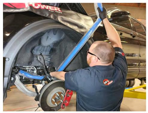
10F It is extremely difficult to spread open the front bushings to install on the bar. Instead, it is easier to just insert it from the end and slide it into place.
