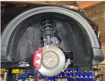
2F Remove the front undertray by removing the array of screws using a 7mm socket, including a few push clips.
