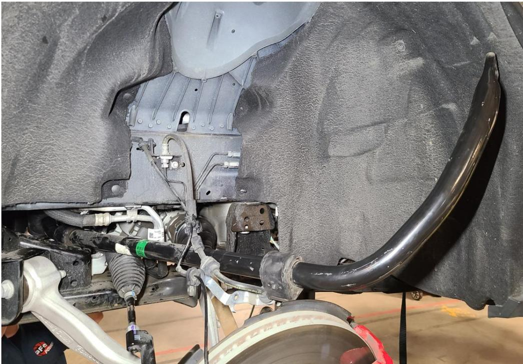
With the ends pointing up, the sway bar can sneak along in front of the engine.
