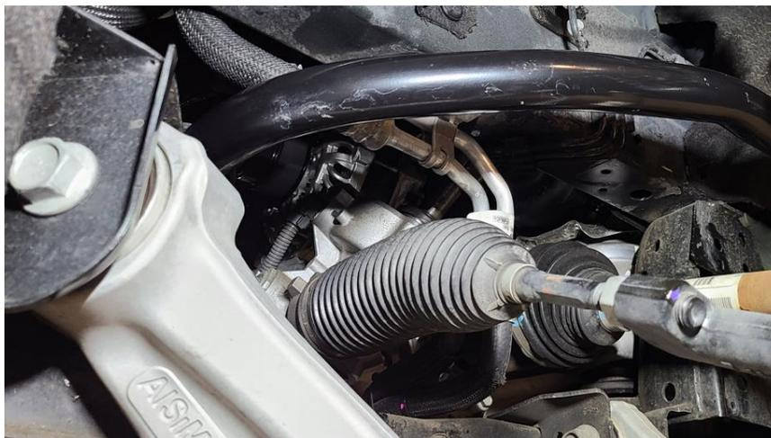
4F Undo the end links from the sway bar ends using a Torx T45 socket and 21mm wrench.
