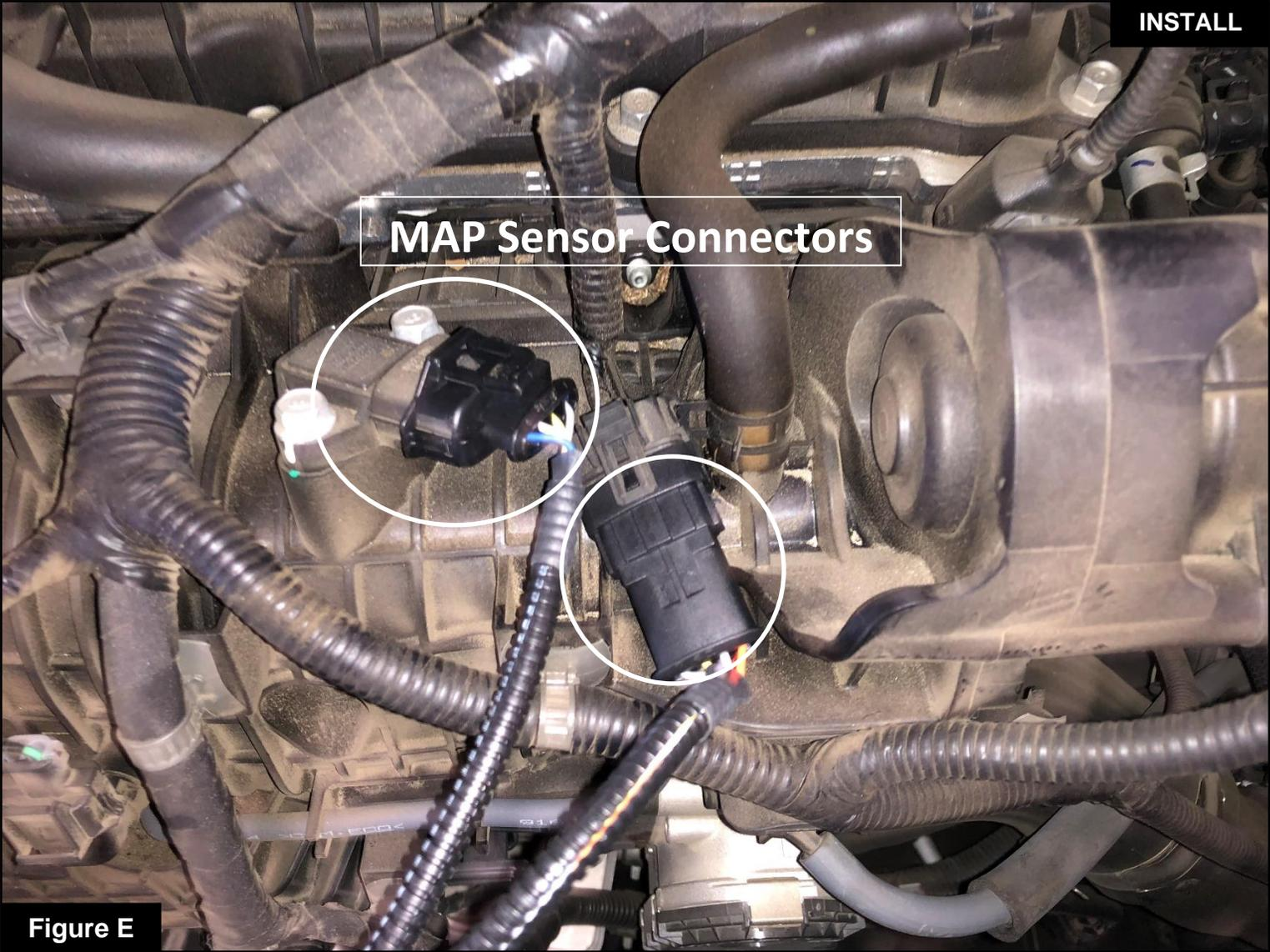
**MAP Sensor Connectors****Figure E****Refer to Figure E for Steps 7-9**
