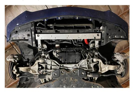
3F Disconnect the end links from the stock sway bar using a 19mm wrench for the stud and 17mm socket for the nut.
