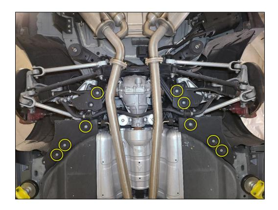
3R To gain more clearance when removing the sway bar, unbolt the exhaust hanger brackets and center brace with a 12mm socket to drop the exhaust system low enough for passage. Use a jack or jack stand to support the exhaust as it hangs down.
