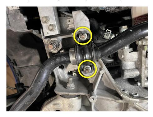
5F Remove the factory sway bar from the vehicle. Note the orientation of the sway bar when removing. (i.e. observe which is the top of the sway bar and how the ends are pointing.)
