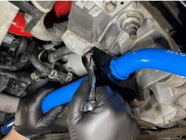
PF Reattach the end links to the sway bar ends reusing the factory nuts. The hole closest to the end is the softest setting. Settings get stiffer as you move away from the ends. (optional: apply thread locking compound to the end link thread)
