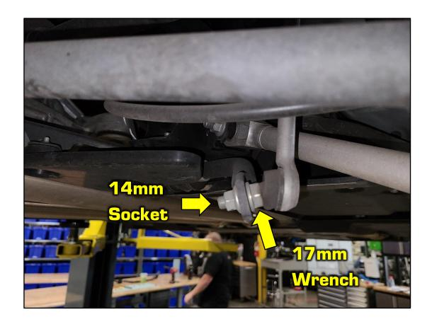
5R Undo the sway bar bushing brackets. (14mm socket)
