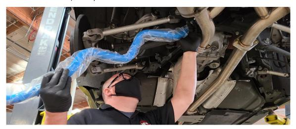
Install bushing onto the sway bar. The bushings should be positioned just inside of the centering rings. Slide the aFe Control bushing bracket onto the bushings and mate the sway bar assembly to the subframe. Reuse the factory bolts to secure the brackets to the subframe. Fully tighten this hardware to factory specs.
