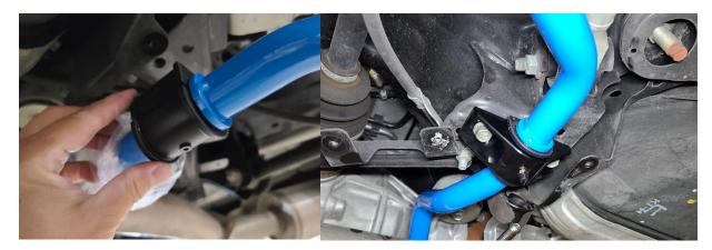
11R Reattach the end links to the sway ends reusing the factory nuts. The hole closest to the end is the soft setting. Settings get stiffer as you move away from the ends. (optional: apply thread locking compound to the end link thread)
