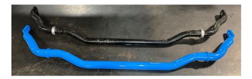
7F Grease the front bushings with the supplied silicone lube and install bushings onto the sway bar. The bushings should be positioned just INSIDE of the centering rings.
