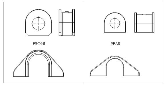
Install the front aFe Control sway bar in the same manner as factory removal. Slide the aFe Control bushing bracket onto the bushings and mate the sway bar assembly to the subframe. Reuse the factory nuts to secure the brackets to the subframe. Fully tighten this hardware to factory specs.
