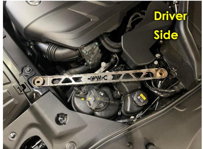
4. Install all (4) M10 bolts with washers by hand first. Then torque down the bolts to **30 ft · lbs** with a 12mm socket and you're done.
