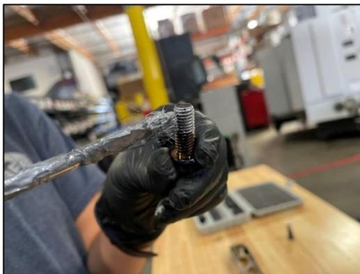
*(Optional) Apply anti-seize onto the first half of the bolt threads.*
