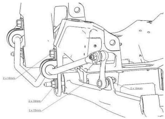
Using a 15mm box end wrench and an 18mm socket and ratchet remove the two lower nuts and two upper bolts from the sway bar bushing bracket. Remove the sway bar and end link assembly.
