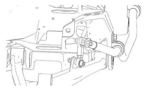
Attach the end links to the sway bar. (Adj. end links shown. Not included)
