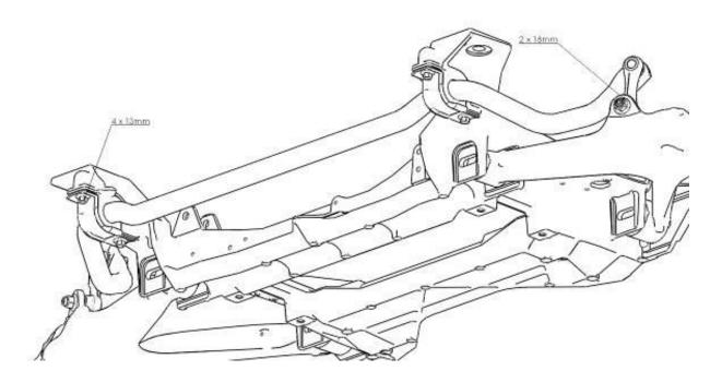
Remove the four 18mm bolts attaching the sway bar bushing brackets to the subframe. Remove sway bar and end link assembly.
