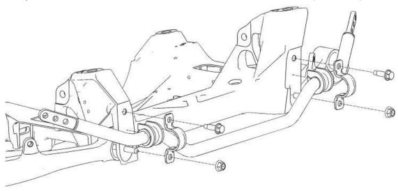
Install the front end links to the rear control arms as shown. It is not necessary to tighten the jam nuts on the end links at this point. See Initial Setup for end link adjustment.
