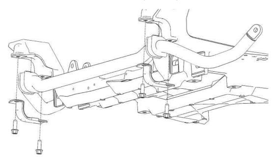
Install the front end links to the front control arms as shown. It is not necessary to tighten the jam nuts on the end links at this point. See **Initial Setup** for end link adjustment.
