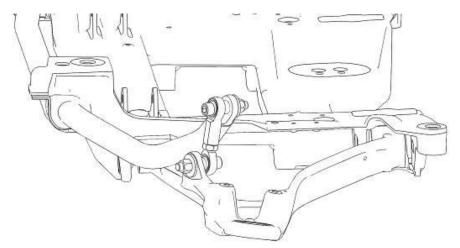
Attach the end links to the sway bar. (Adj. end links shown. Not included)
