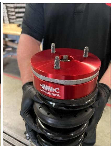
17. Reverse Steps 1 – 11 for reinstallation, torquing all hardware to factory specifications designated in the table below.
