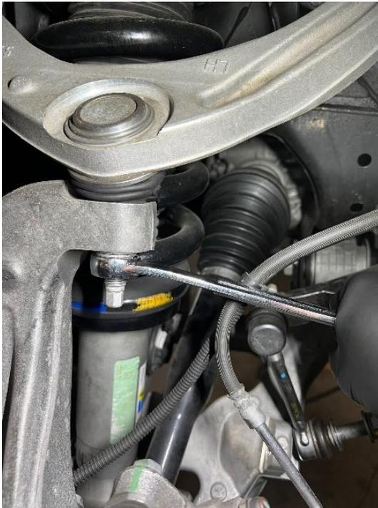
9. Using a 1-3/16" impact socket and wrench, loosen and remove the Lower Shock Eyelet bolt.
