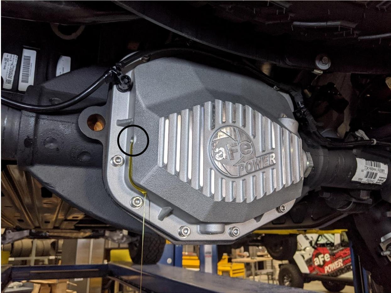
19. Using the top fill port, fill the aFe differential cover with new gear oil. Fill until gear oil runs out of the 1/8" NPT port on the side of the cover (about 4 quarts).
