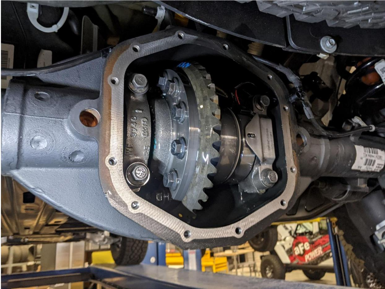
9. Use a clean, lint free rag to wipe down the remaining gear oil from the housing.
