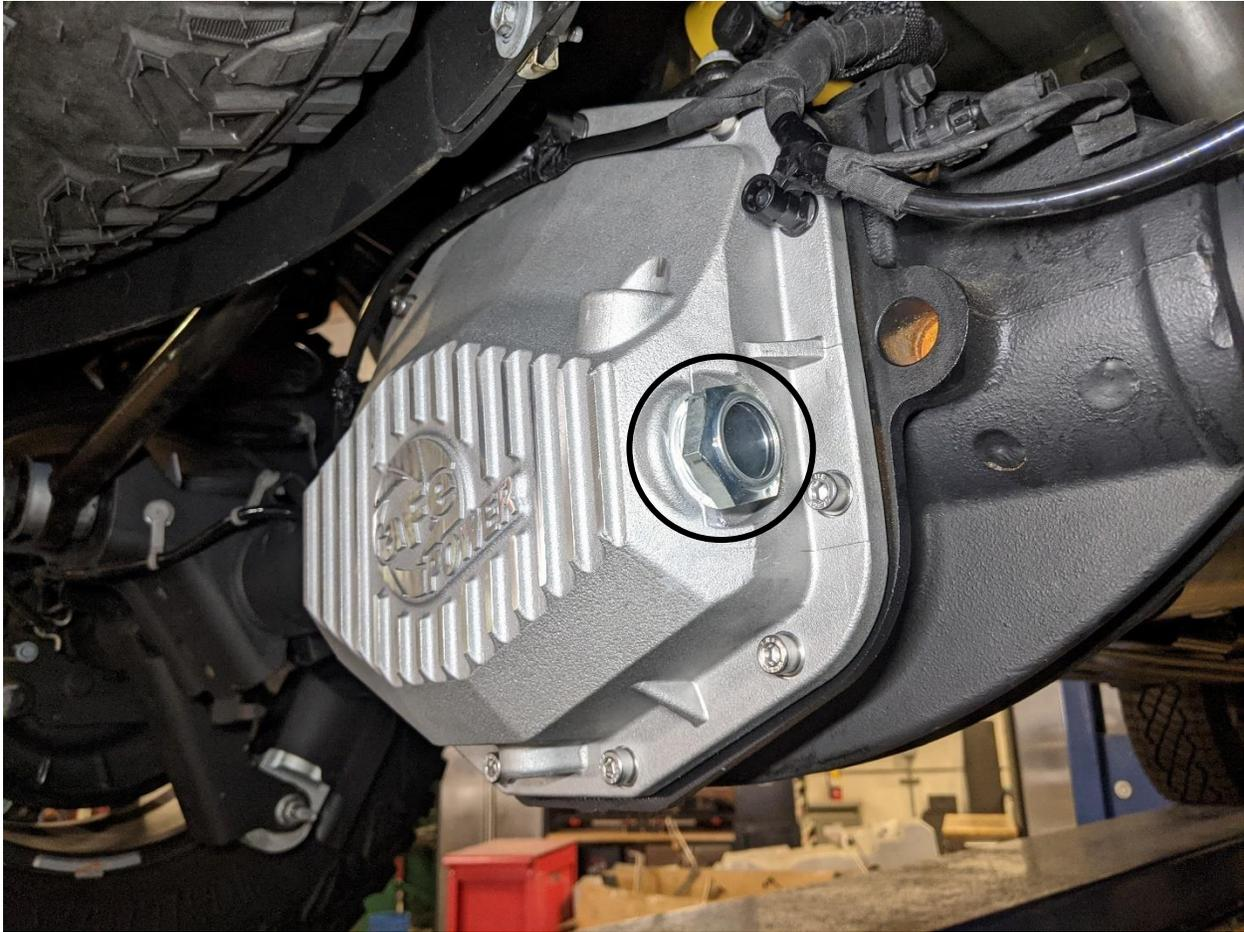
**Note: For all NPT plugs, secure 1.5-3 turns past finger tight. The fitting should never bottom out in the port.**
