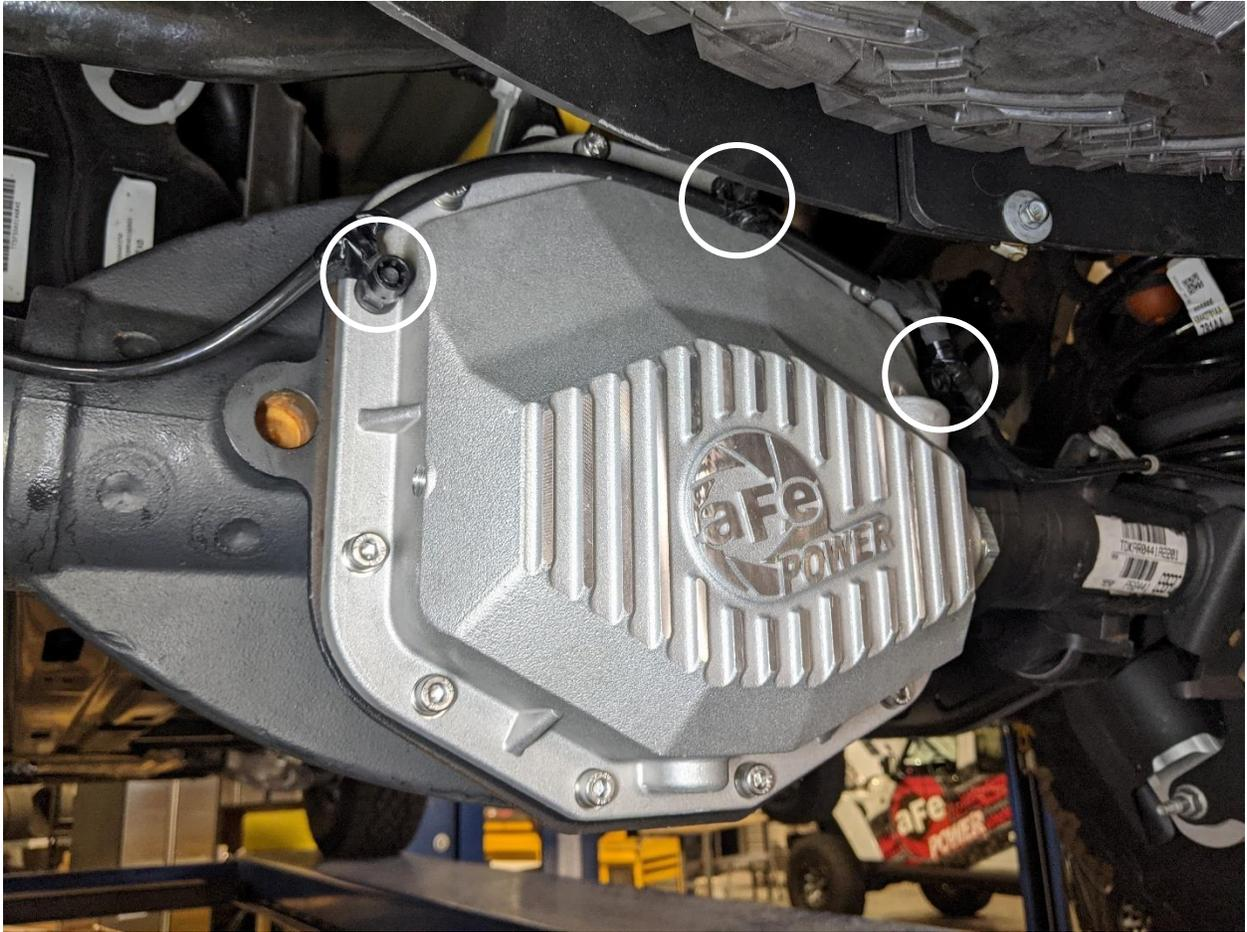
15. Torque all of the mounting bolts to 12-16 ft.-lbs. in a crisscross pattern.
