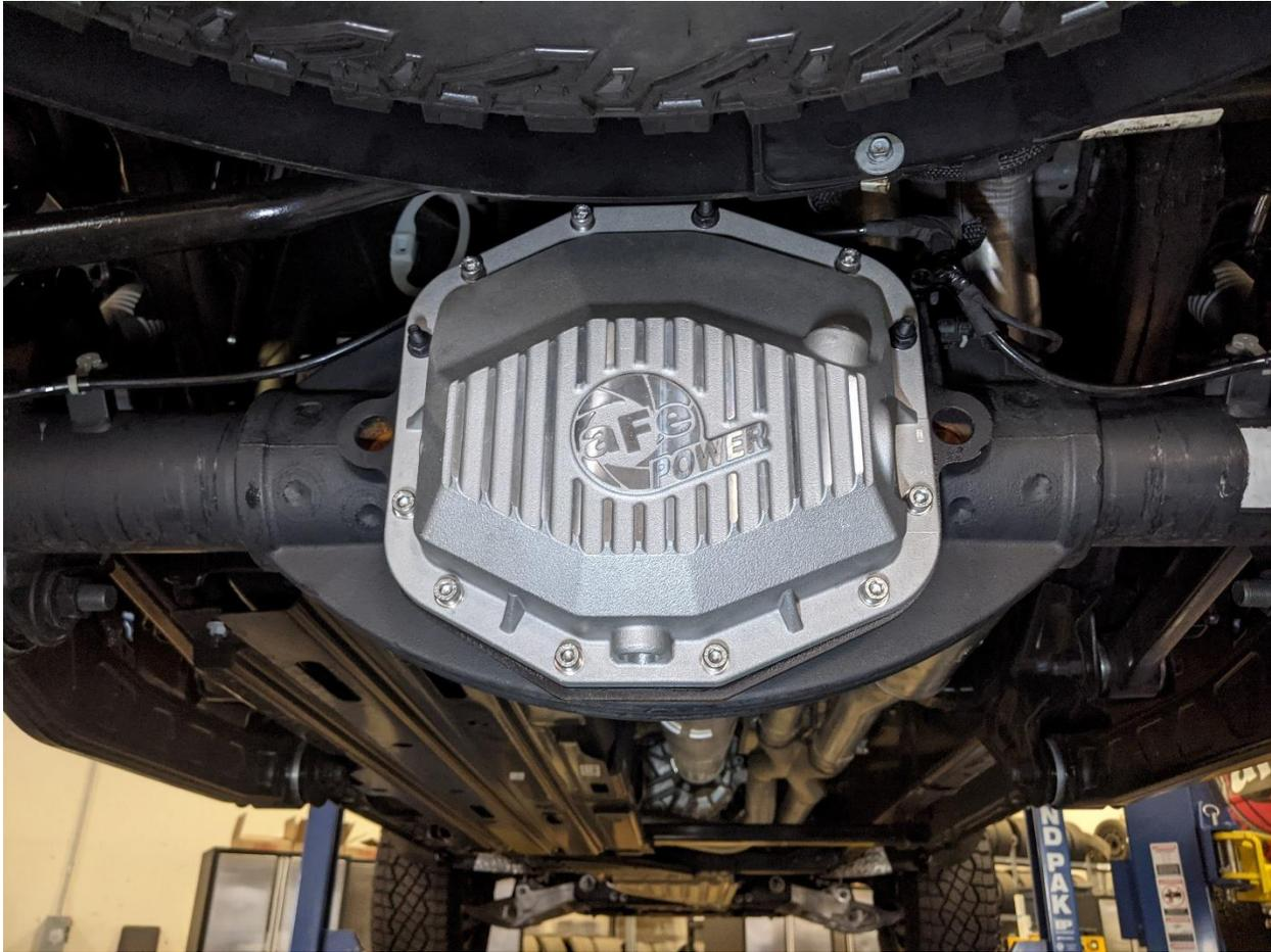
12. Hold the OEM gasket and supplied aFe differential cover into position, aligning the screw holes. Install one (1) of the supplied M8x1.25x25 socket head screws and flat washers at the top of the cover to hold it in place.
