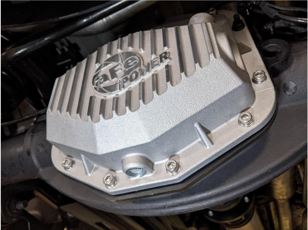
17. Install the supplied M12x1.25 drain plug and crush washer into the bottom of the cover (secure about  $\frac{1}{2}$  turn past finger tight).
