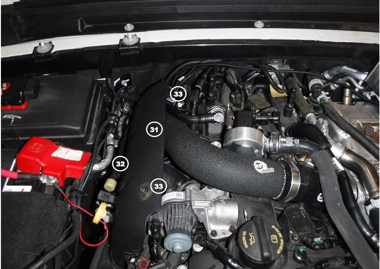
36. Reinstall the side engine cover into the vehicle (31)
