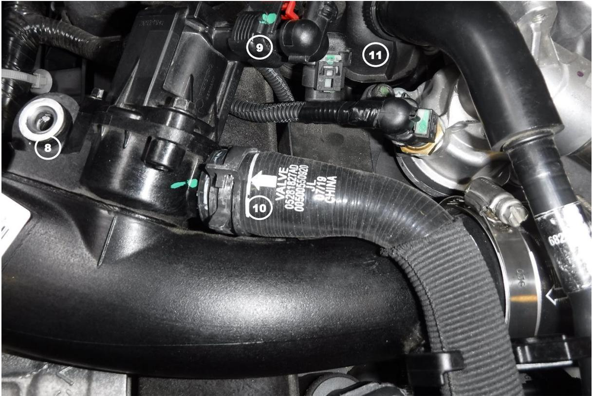
9. Remove the screw securing the charge pipe to the vehicle (8)
