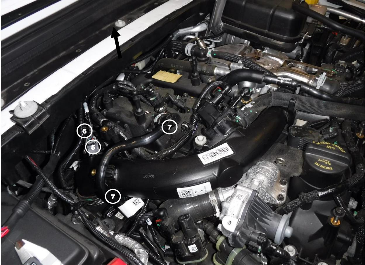
6. Release the security tab on the MAP sensor connector, then disconnect it from the charge pipe ⑤
