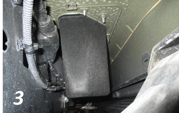
13. In the engine compartment zip tie the control box along the wire harness on the passenger side of the vehicle. Run the wire ring terminals in the wire harness crossing the fire wall to the battery and run the rest of the wire down the back of the firewall to meet the rest of the wire harness. Use the provided zip ties to secure the wire. **(You will need to use the provided wire extensions.) Refer to FIG 4 & FIG 5.**
