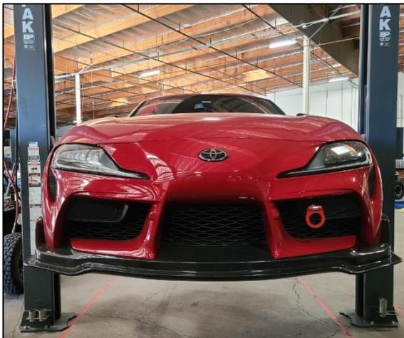
2F Remove the front wheels with a 17mm socket.
