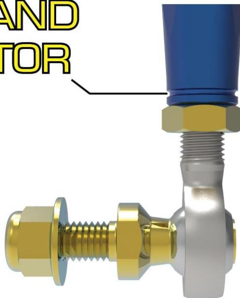
6F Install the end link in the same manner as stock removal. Install the left-hand (tightened) end on the strut and right-hand end on the sway bar end
