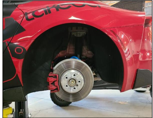
3R Unfasten the left end link from the car using a T30 socket to hold the studs and a 16mm wrench to undo the nuts.
