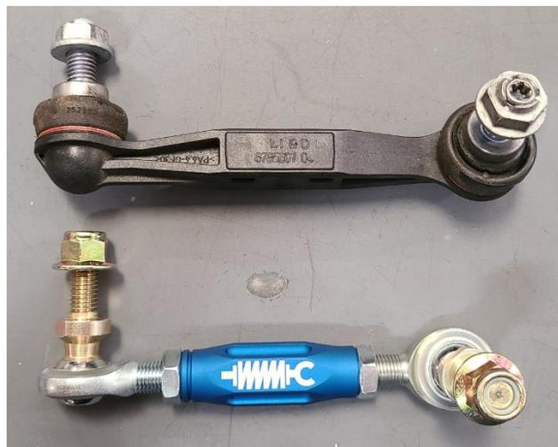
Optional: For cosmetic purposes, to avoid scratching the blue anodizing on the sleeve, we suggest using an aluminum adjustable wrench or applying masking tape to a normal wrench. The sleeve size is 3/4" and the jam nuts are 11/16".
