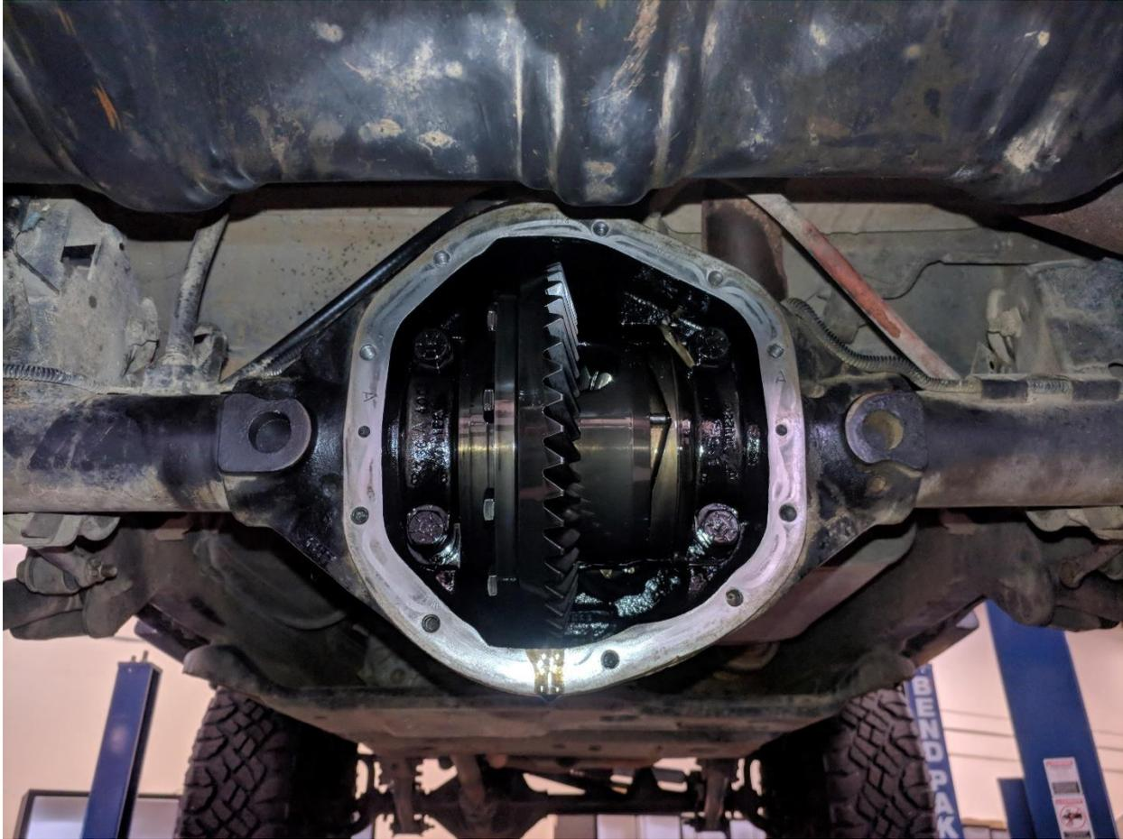
6. Allow all of the gear oil to drain from the differential.
