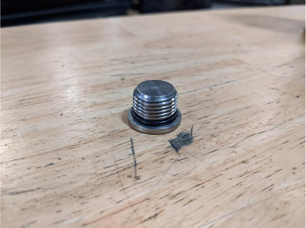
19. Apply gear oil to the provided -016 O-Ring, then install it on the provided M18x1.5 plug.
