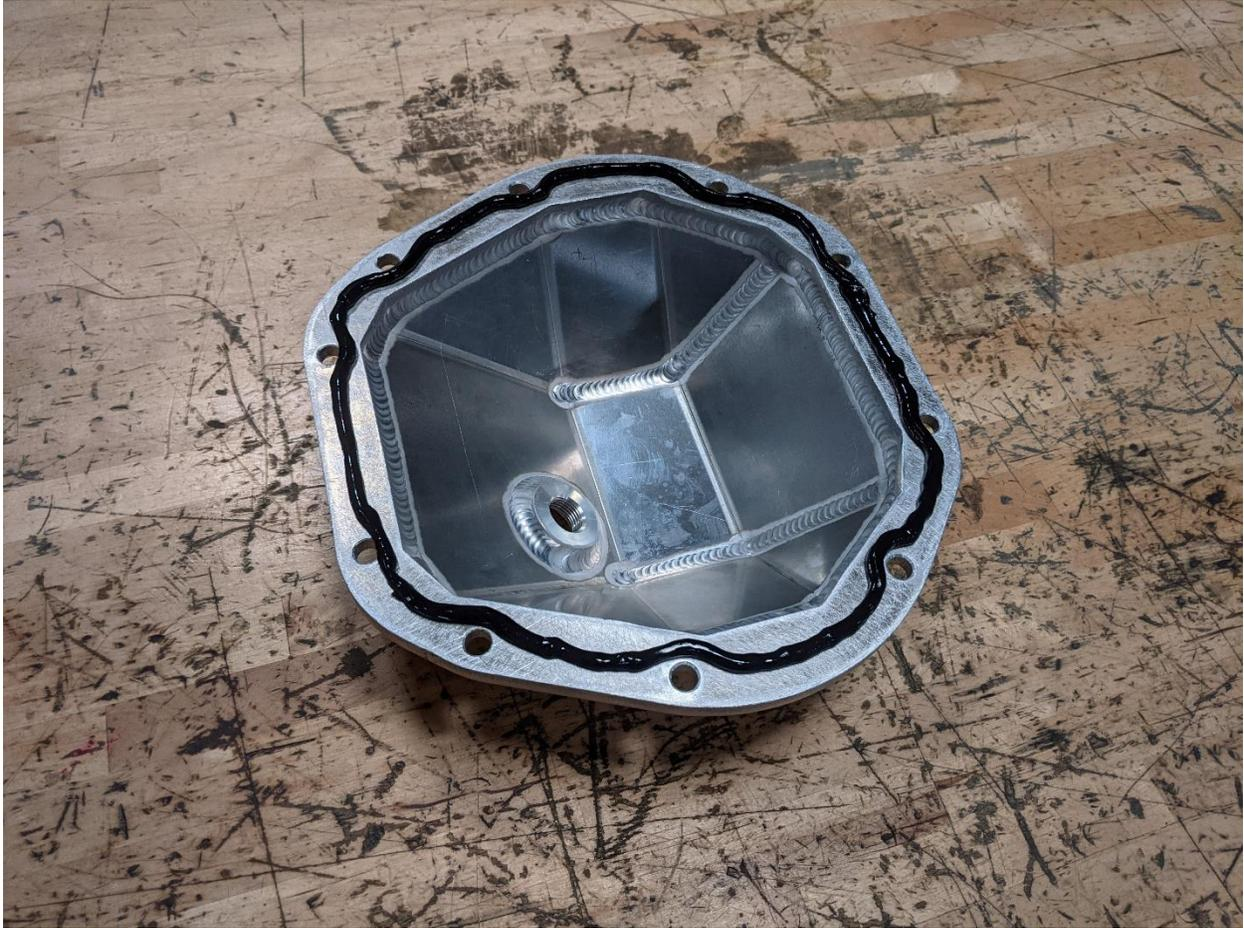
12. Hold the supplied aFe differential cover up to the gasket surface to make sure you will be able to maneuver it into place easily.
