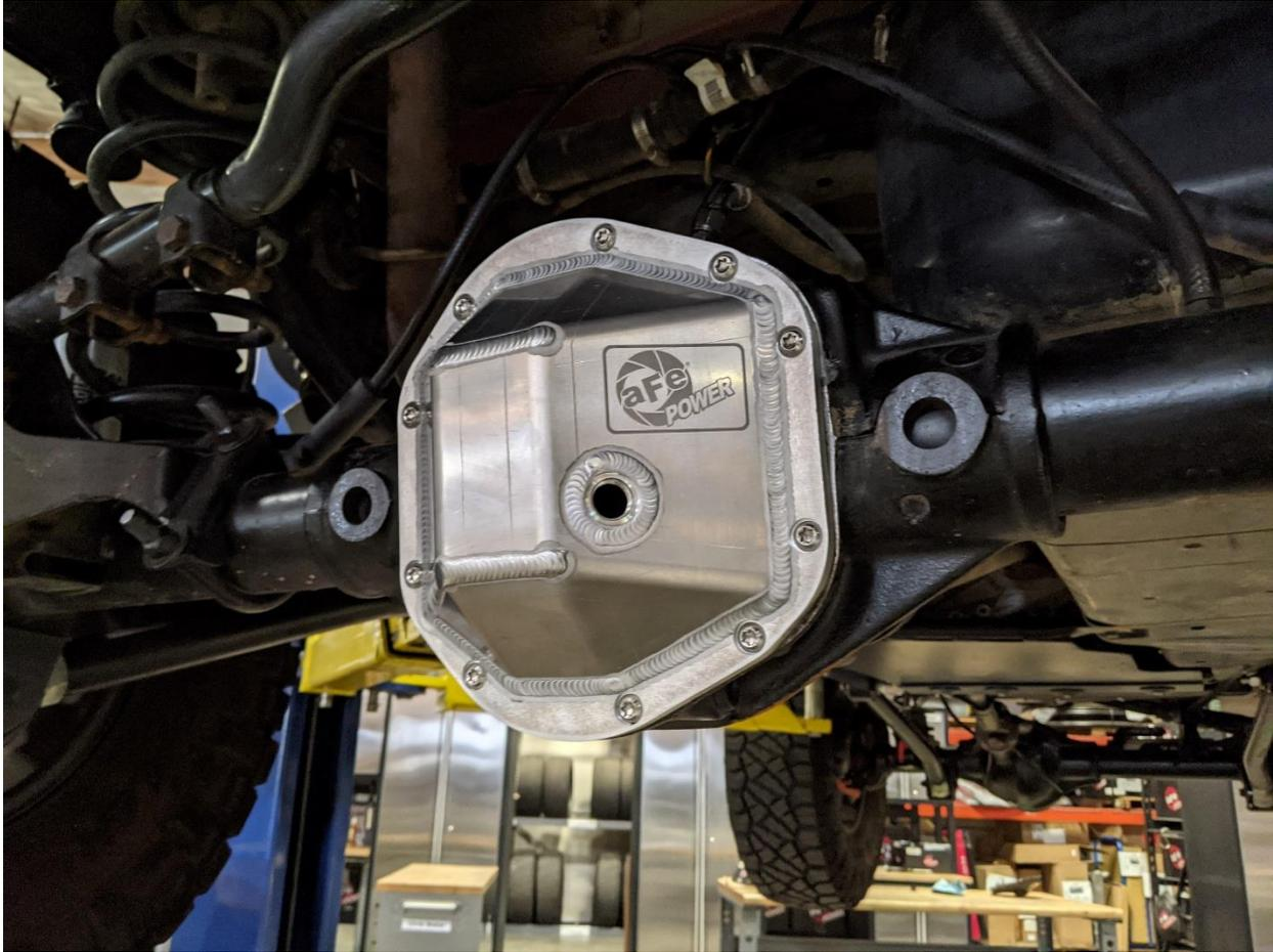
14. Hold the aFe differential cover into position, aligning the screw holes. Install four (4) of the supplied 5/16-18 x 3/4" button head screws and flat washers into separate sides of the cover to hold it in place.
