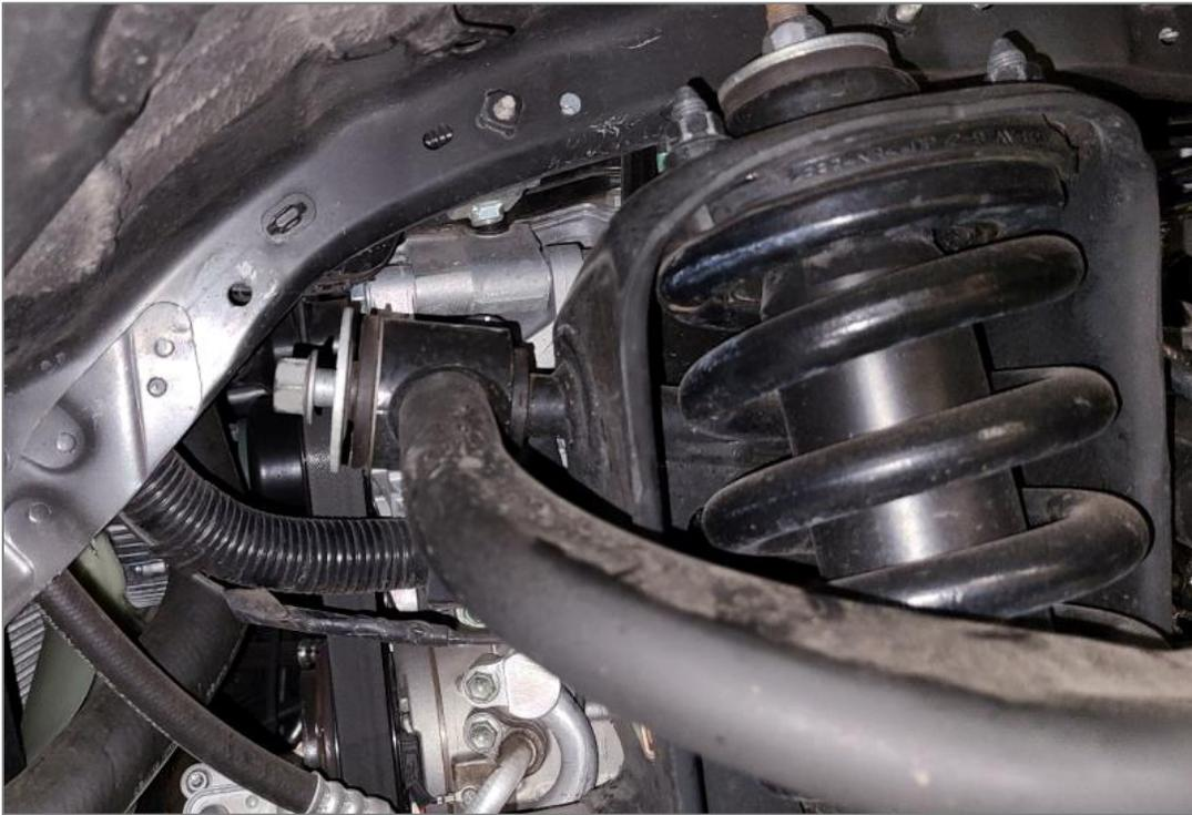
Cut the bolt head off and slide the bolt towards the back to remove.
