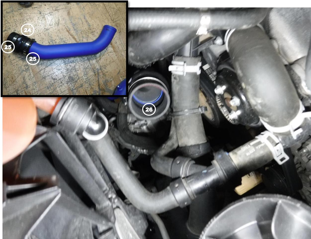
35. Install the last 2-1/2" x 5.5"L aFe hump coupling (24) onto the less angled side of the smaller intercooler tube along with one of the 2-5/16" – 3-1/4" clamps on each end of the coupling, (25) do not tighten the clamps yet.
