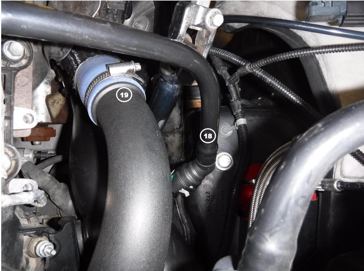
25. Rotate the vent tube (18) from the turbo inlet tube out of the way.
