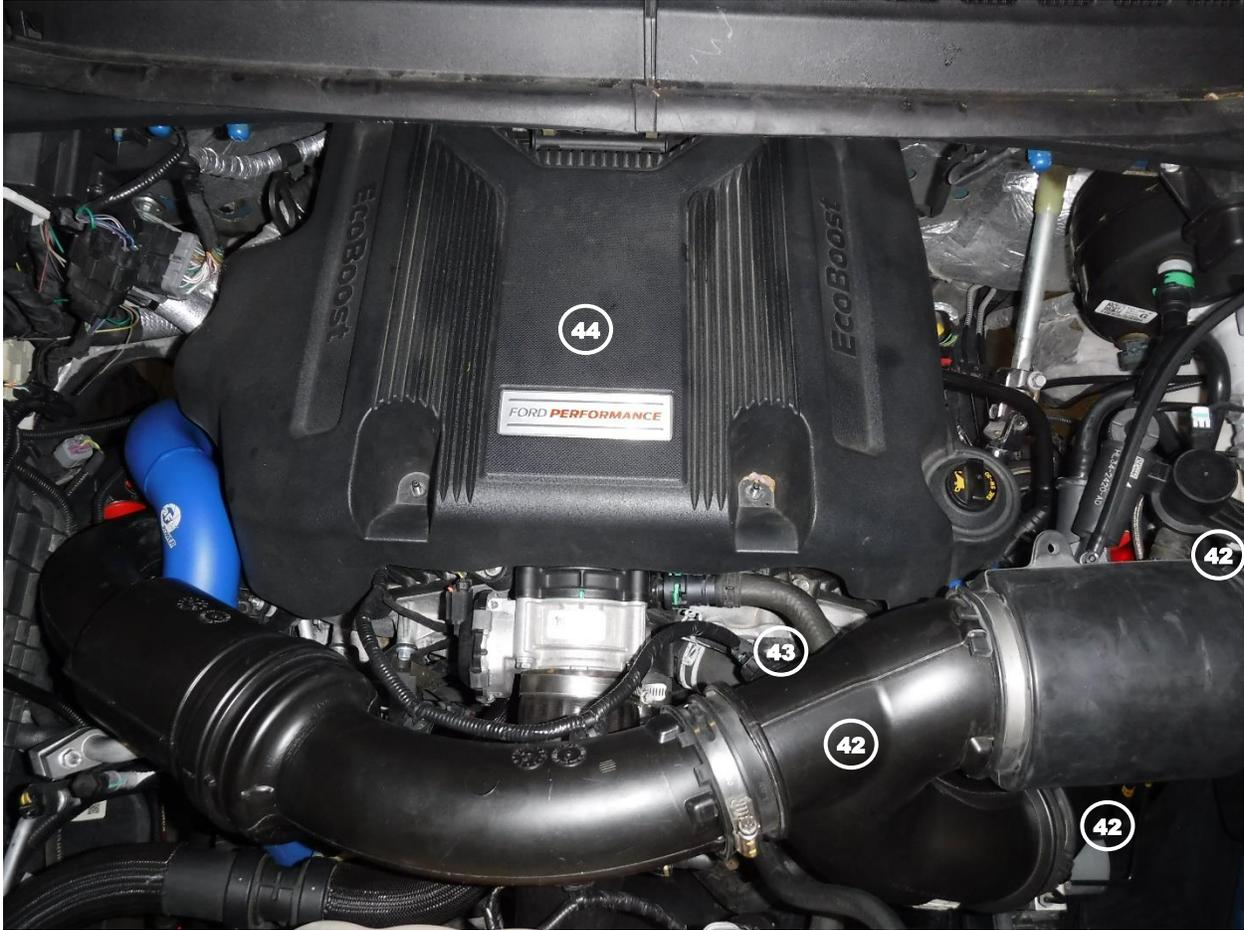
52. Reinstall the intake tube y-bridge and tighten the clamps (42)
