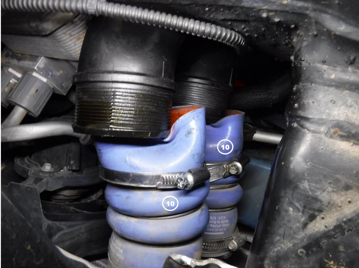
14. Loosen the clamps securing the hot side intercooler tubes (10) to the intercooler on the passenger side of the vehicle.
