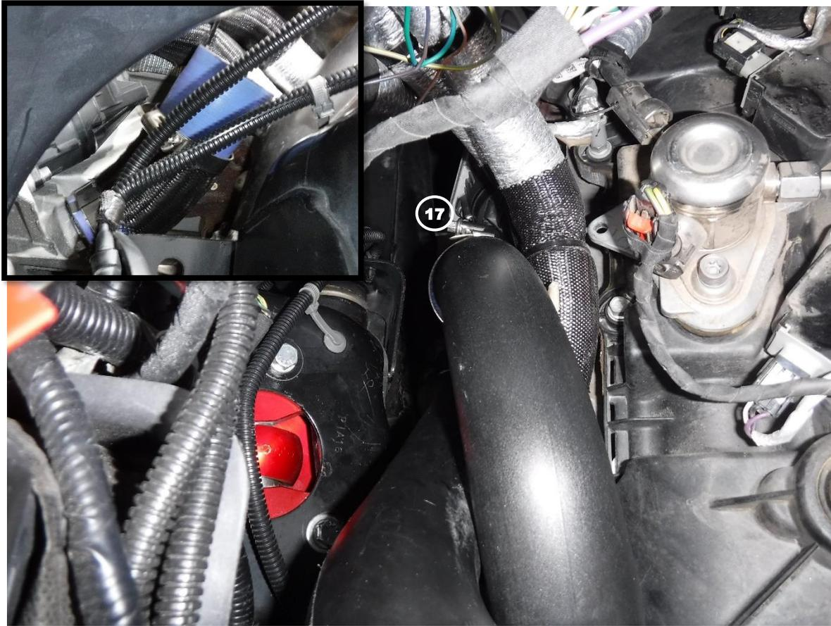
22. Loosen the clamp (17) securing the hot side intercooler tube to the turbo coupling on the passenger side of the vehicle and disconnect it from the coupling.
