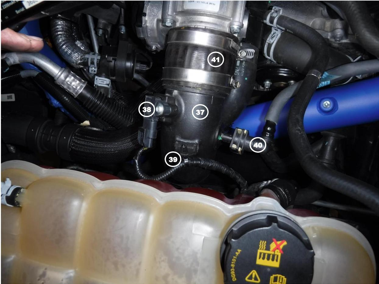
**Note: Be sure to thoroughly clean all oil residue off of the connections before installing the supplied aFe couplings onto the vehicle**
