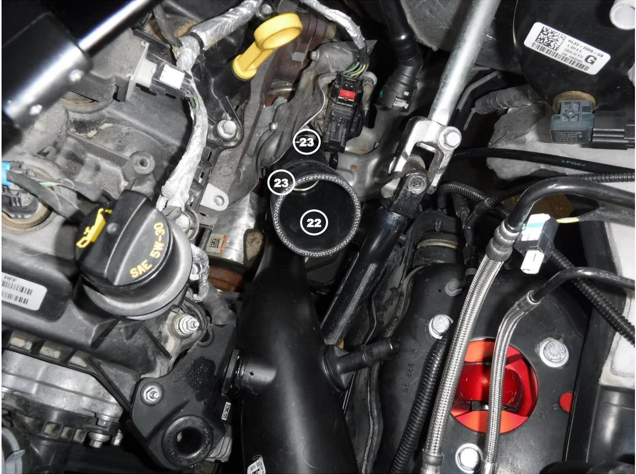
33. Install the 2-1/2" x 1-3/4" x 15° aFe reducer coupling (22) onto the driver side turbo along with one of the supplied 1-9/16" -2-1/2" clamps , do not tighten the clamp yet.
