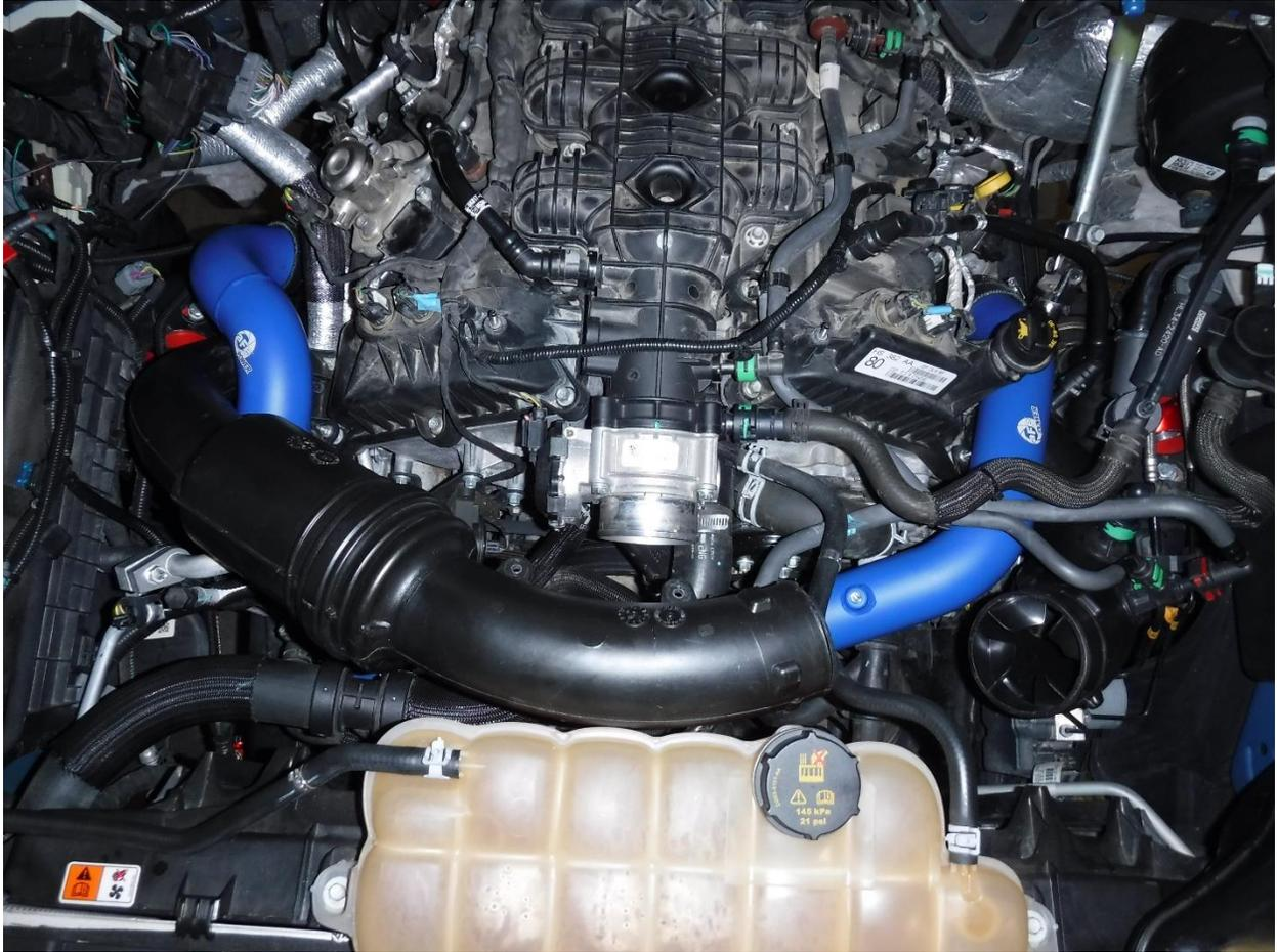
44. Ensure the aFe hot side intercooler tubes are not touching anything and tighten all of the clamps.
