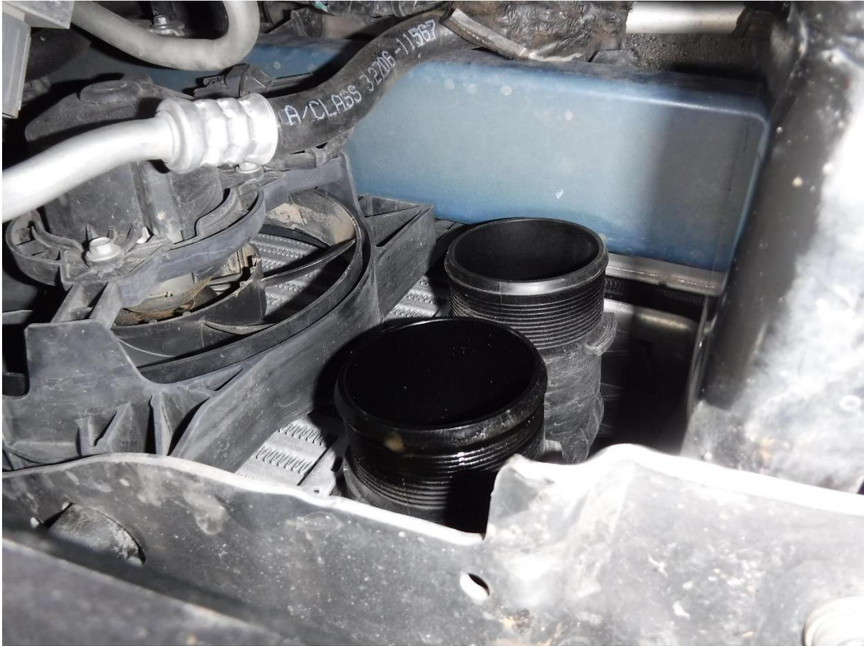
29. Loosen the two (2) clamps securing the factory hot side intercooler couplings onto the intercooler on the passenger side of the vehicle.
