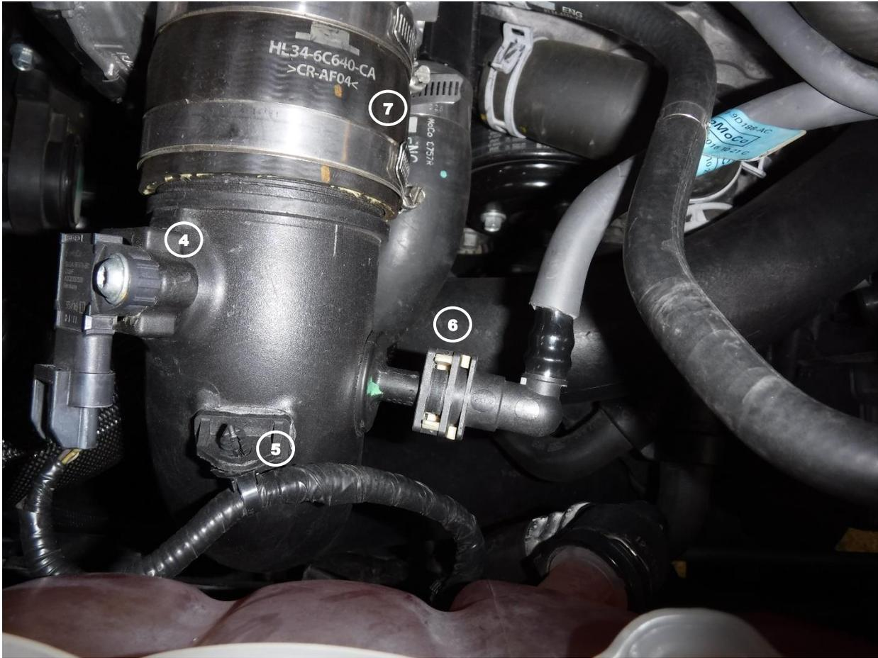
6. Disconnect the electrical connection ④ from the cold side intercooler tube.
