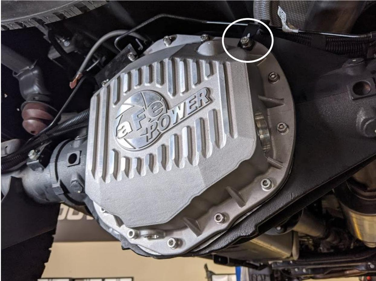
17. If applicable, reinstall the brake line cable retention pad using one (1) M8x1.25x40 socket head screw, one (1) spacer, and two (2) flat washers.
