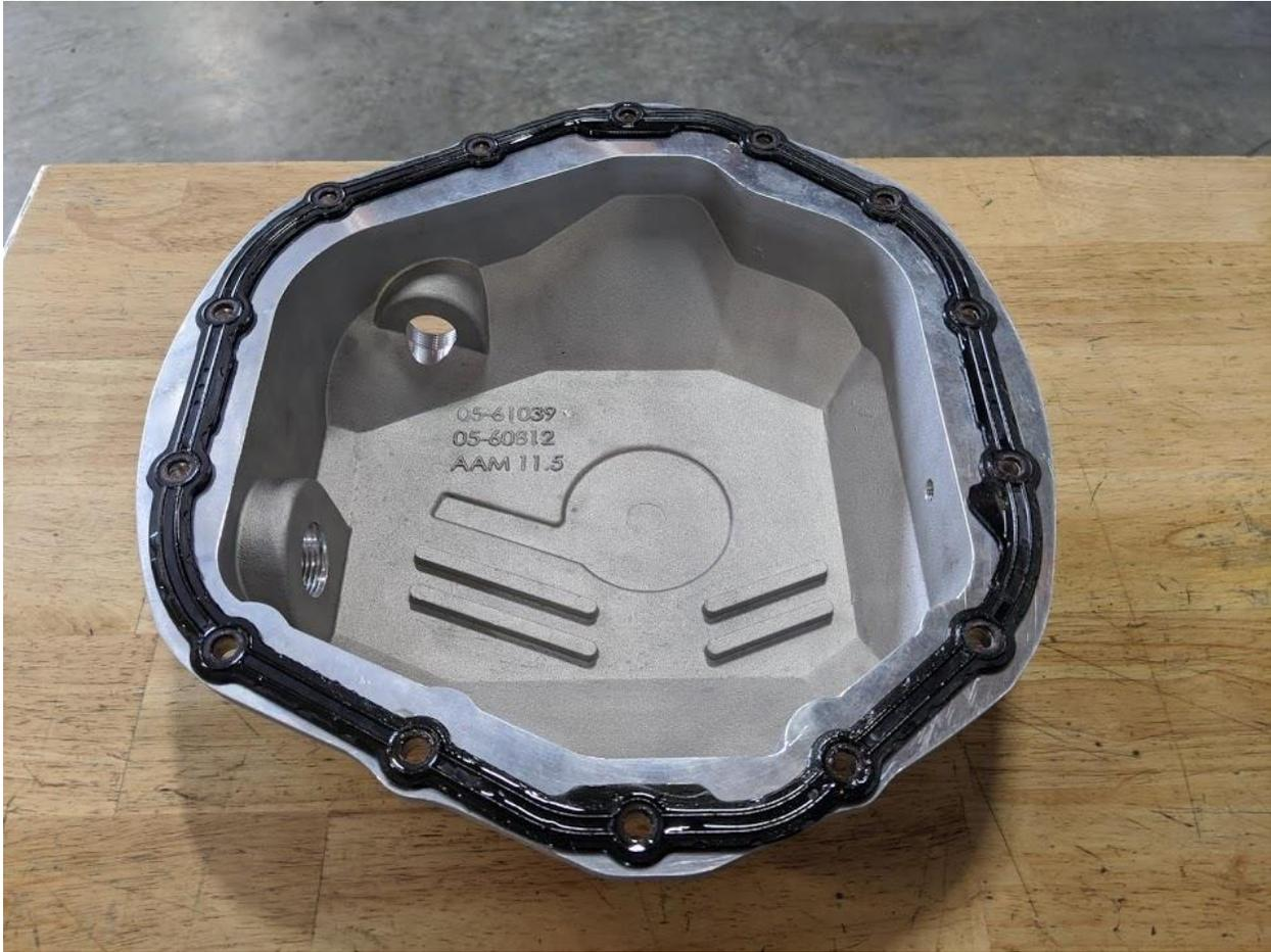
14. Line up the gasket removed in Step 10 to the supplied aFe differential cover.
