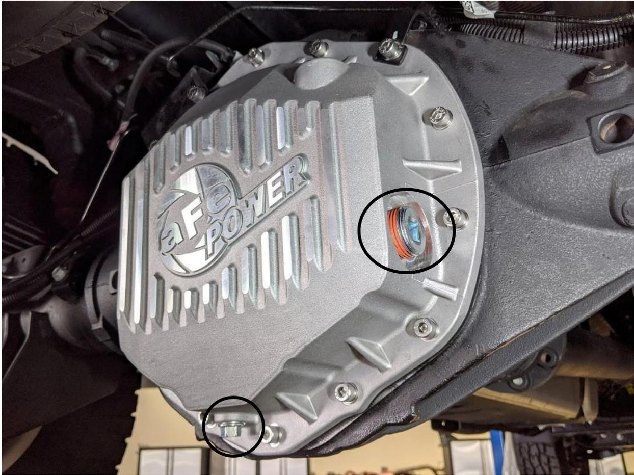
20. Install the supplied M12x1.25 drain plug and crush washer into the bottom of the cover.
