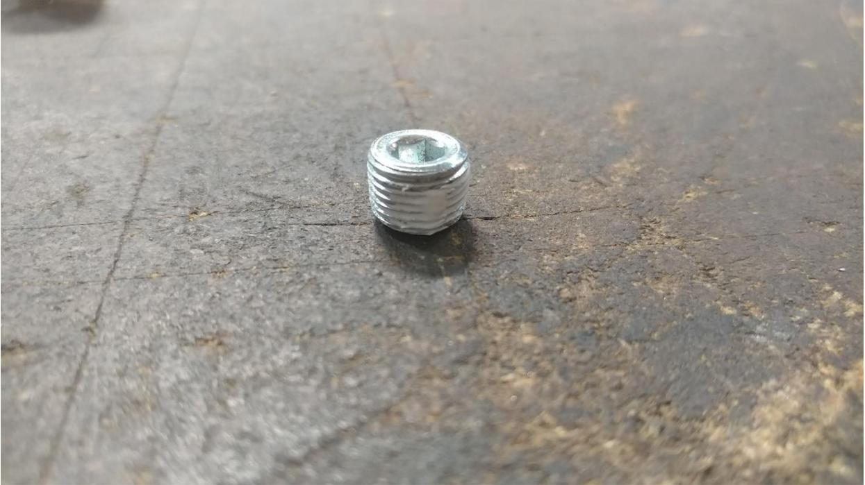
22. Apply Teflon pipe sealant to the threads of the supplied 1/8" NPT plug.
