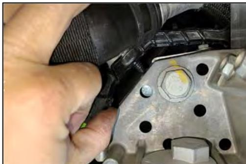
17F Unbolt the steering rack from the subframe using a 15mm socket and wrench on the (2) bolts & nuts.
