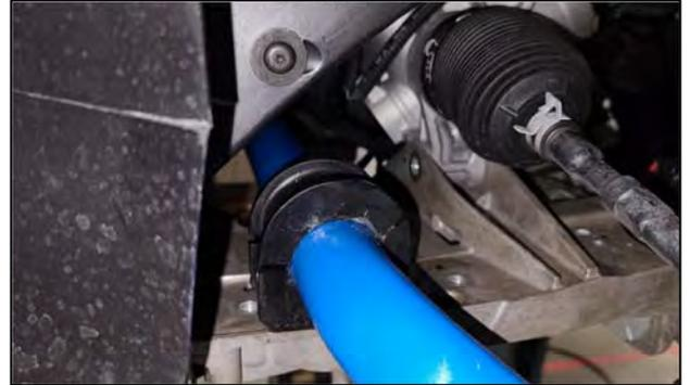
28F Install the billet bushing brackets onto the bushings with the 90° zerk fittings facing out.
