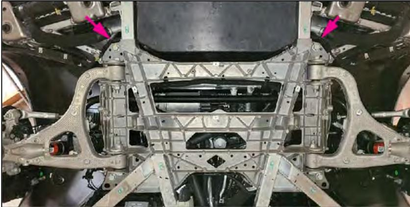
When attaching the end links back onto the aFe Control sway bar, you have 3 position options. The hole closest to the end is the softest setting. Refer to the chart at the end of this document for more details.
