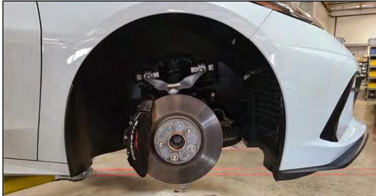
3F Remove the front splitter lip. Use T15 torx socket to remove the (21) screws.
