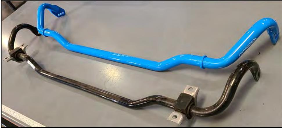
6R Lube the inner surface of the bushings with the provided silicon grease.
