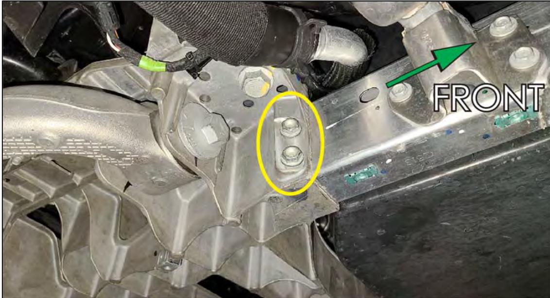
There is a small triangulated bracket that needs unbolting using a 10mm socket. Repeat on other side.
