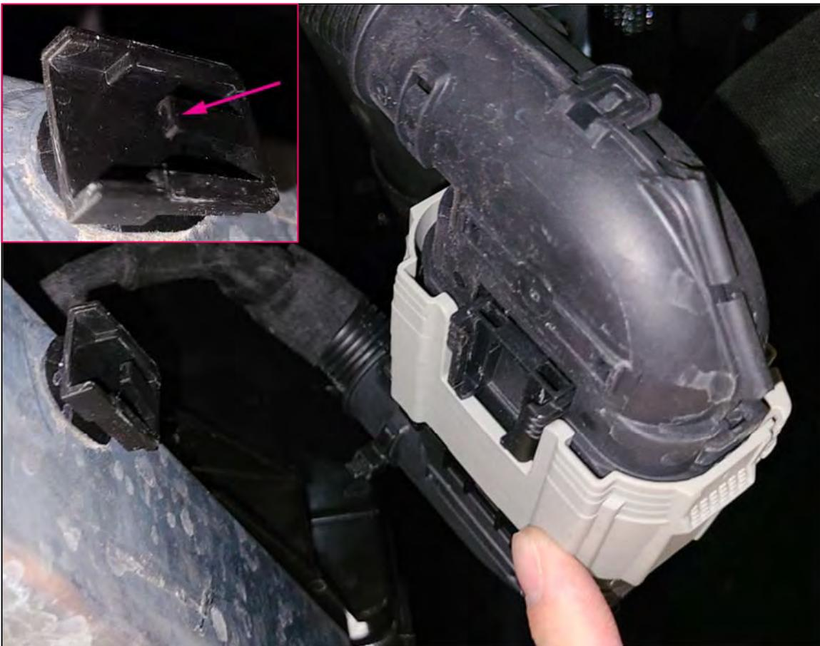
Some clips are attached on the top surface of the subframe that hold the brake lines. Just push the line out of the clip.
