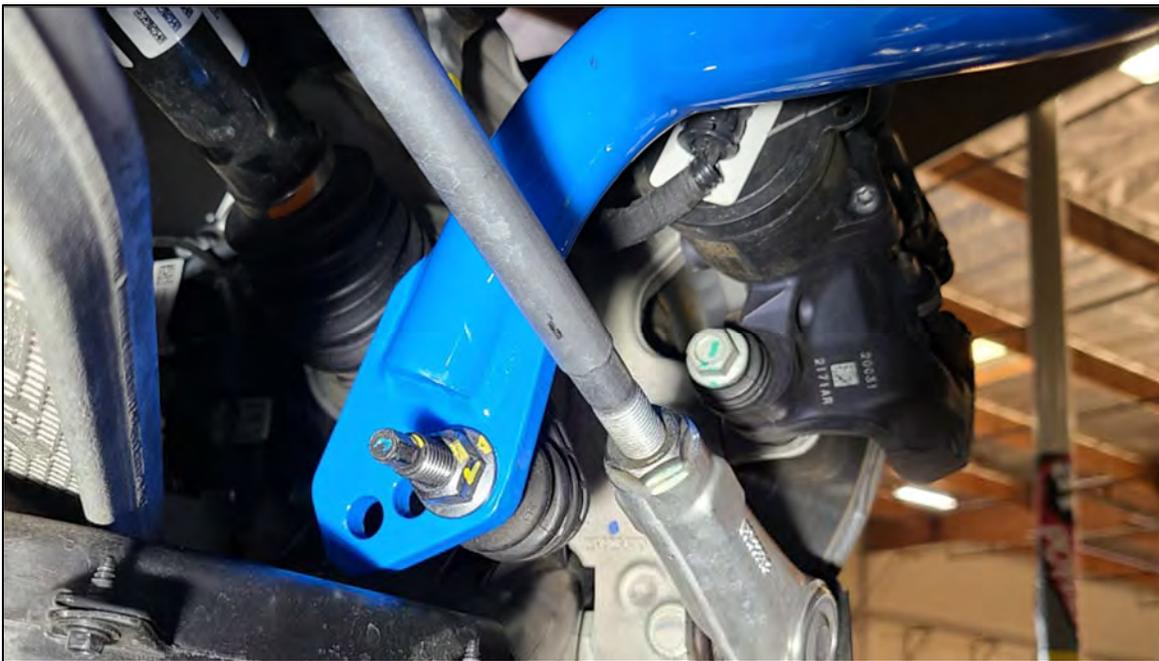
When adjusting to different holes, it is easier to loosen the upper portion of the end links to allow more movement.
