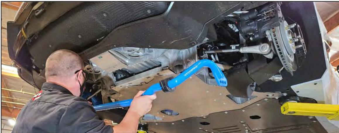
Install the bushing brackets and reuse the factory bolts. Tighten to factory specs.
