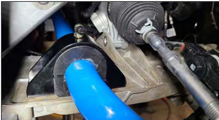
Reuse the factory bolts to fasten the bushing bracket onto the subframe. Tighten to factory specs.
