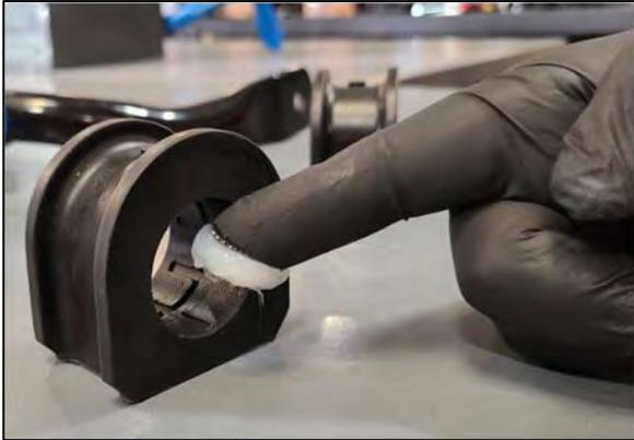
Install the bushings onto the sway bar. The bushings will reside outboard of the sway bar centering rings.
