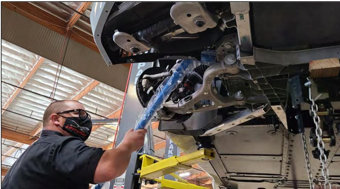
27F Lube the inner surface of the bushings with the provided silicon grease.
