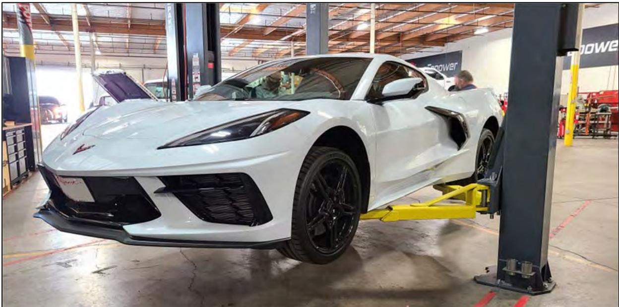
2F Remove the front wheels using a 22mm socket.
