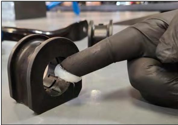
Install the bushing onto the aFe Control sway bar.
