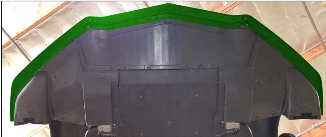
4F Remove the side plastic panels. Use 7mm socket to remove the (2) hex screws and T15 torx socket to remove the (7) screws.
