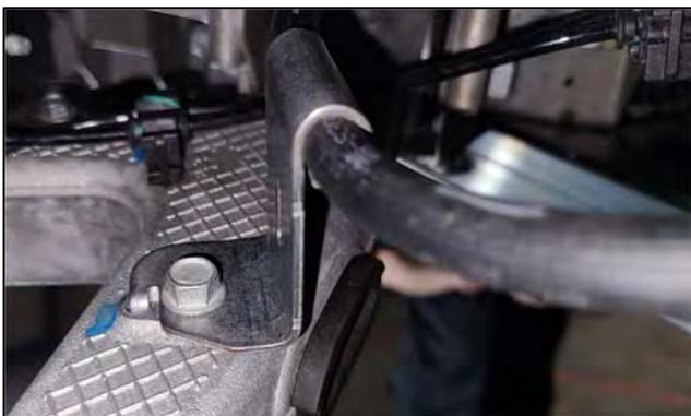
12F Unbolt the brake line/ABS steel bracket with a 10mm socket on both sides of the subframe.
