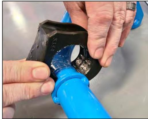
7R Install the aFe Control sway bar in the same manner as removal. It is easier to loosely attach the bar to end links so it can hold the bar for you.
