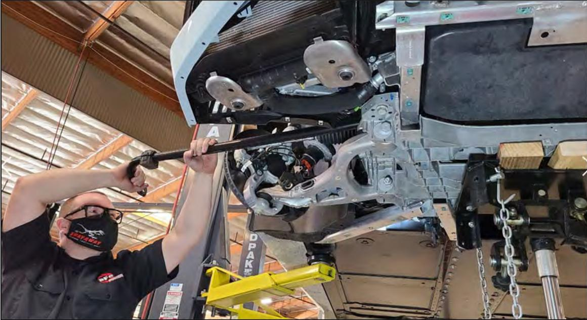
When the bar is almost out, angle the bar downward to remove the final end out. Take care not to damage surrounding components during removal.
