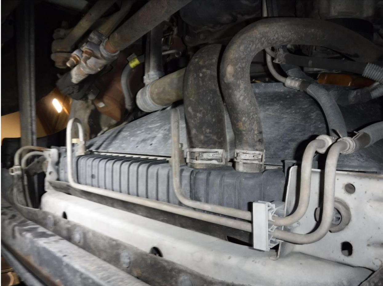
6. Disconnect the lower radiator hose from the radiator.
