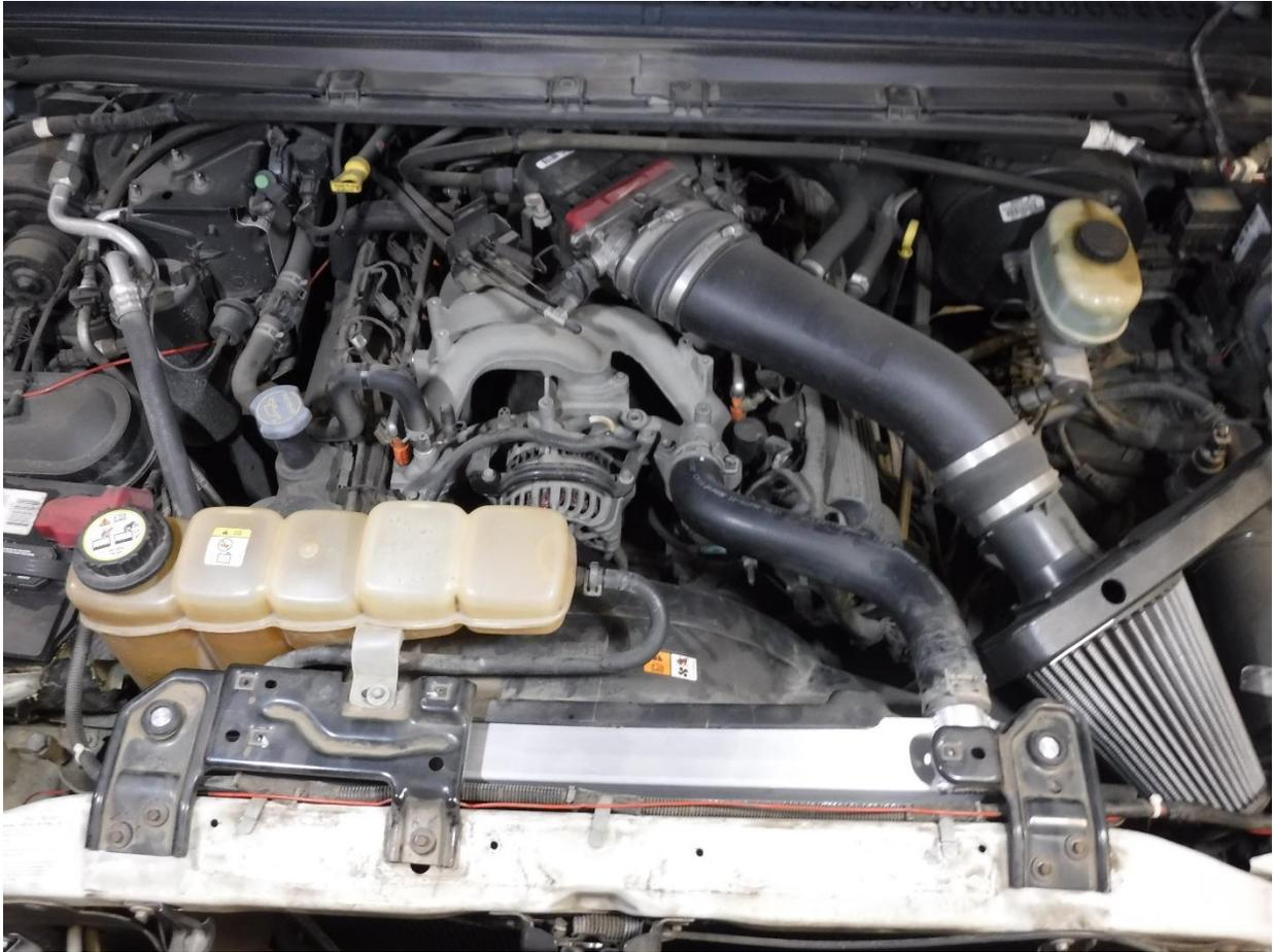
28. Install the expansion tank into the vehicle.
