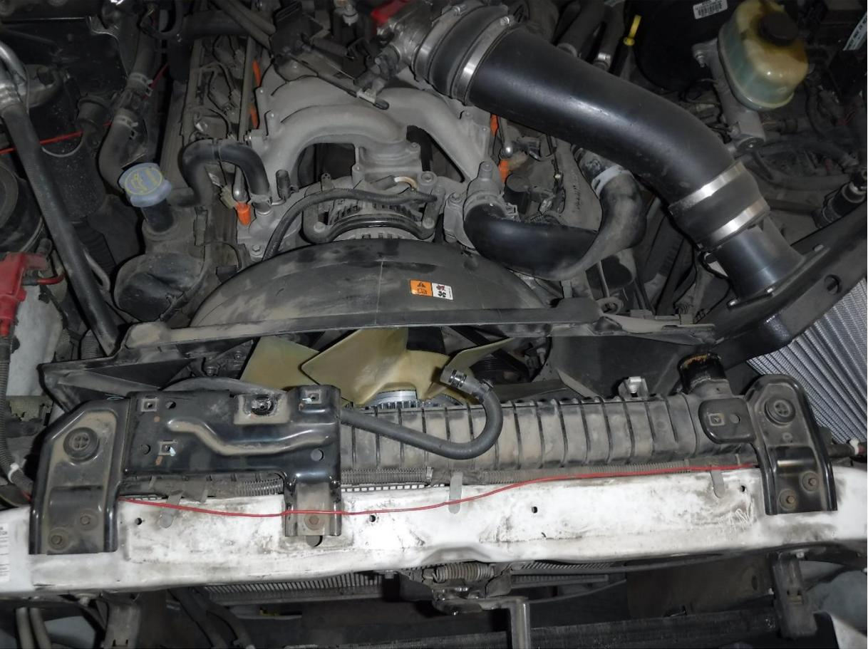
16. Remove the screws securing the two (2) upper radiator mounts to the vehicle.
