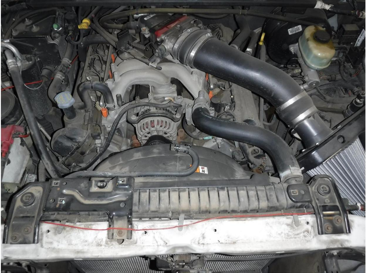
14. Remove the two (2) screws securing the can shroud to the radiator.
