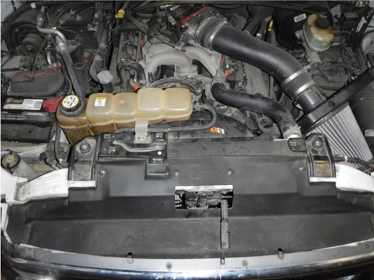
35. Reinstall the rubber cover onto the top of the core support and grille using the factory clips.
