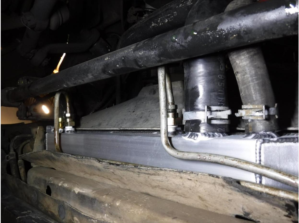
32. Secure the two (2) transmission cooler lines into the fittings on the aFe radiator, be sure the retaining clip is properly clipped in all the way around if equipped.
