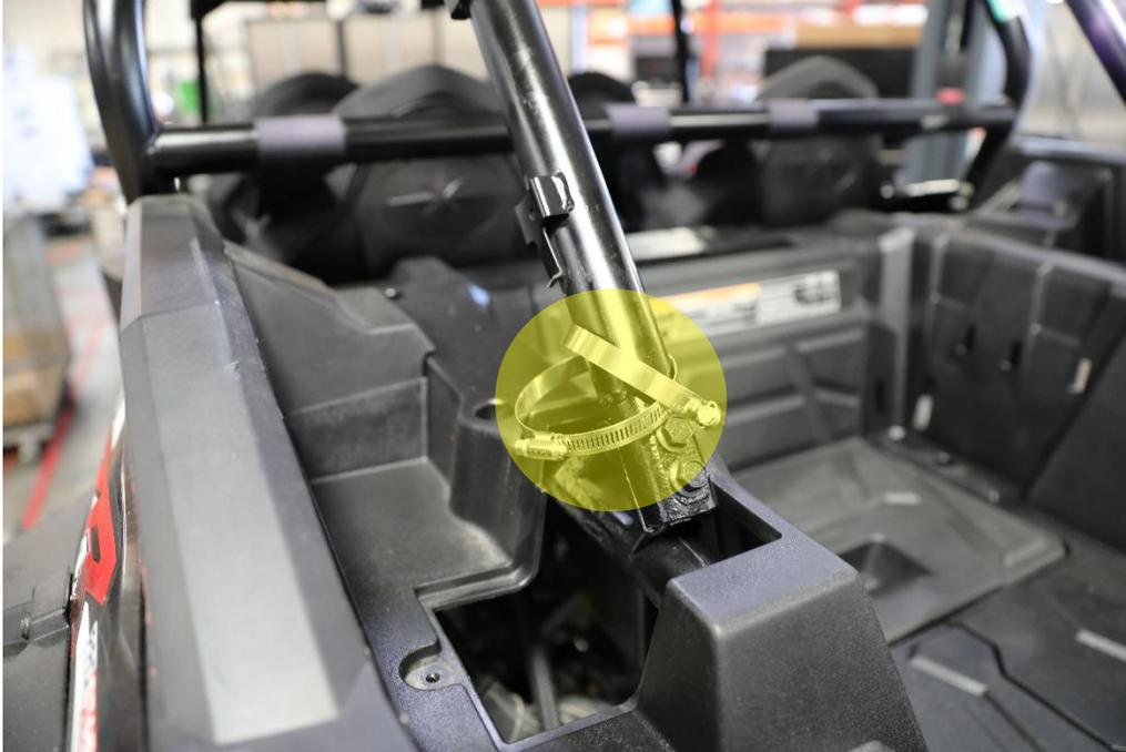
20. Put the reservoir in the location seen below and tighten the hose clamps with the rubber mounts between the reservoir and cage tubing.
