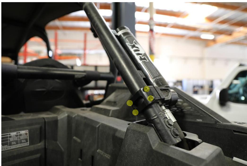
10. Lower the reservoir through the opening and let the reservoir rest where comfortable.
