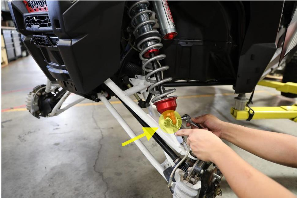
15. Double check that every bolt that was removed has been retightened. Reinstall wheels and tighten lug nuts to factory spec.
