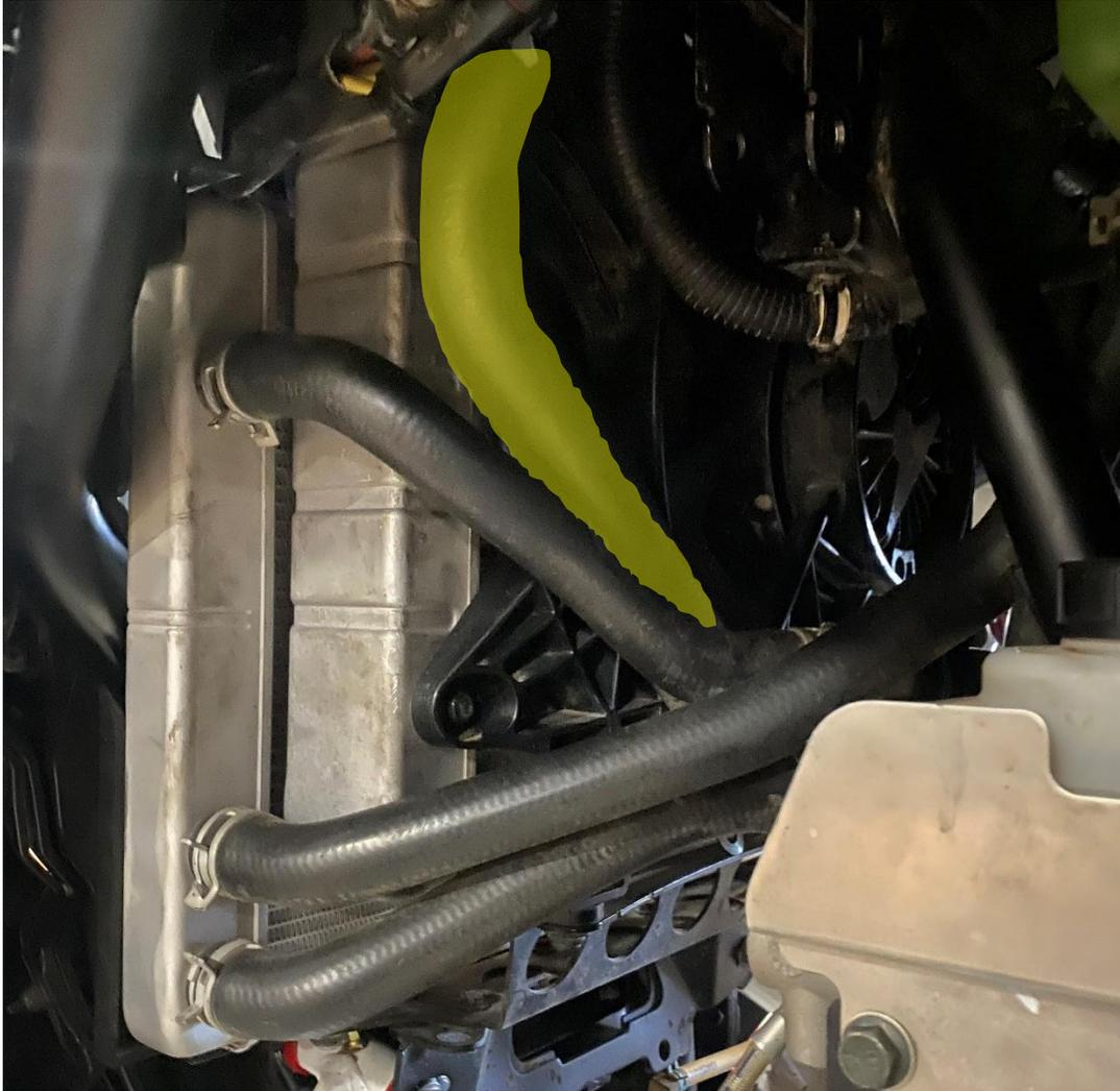
13c. While making sure the radiator hose does not move, re-install the bracket removed from step 13a.
