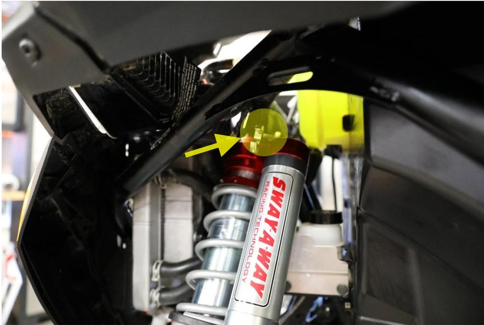
13a. Loosen the 10mm bolt holding on the highlighted bracket.
