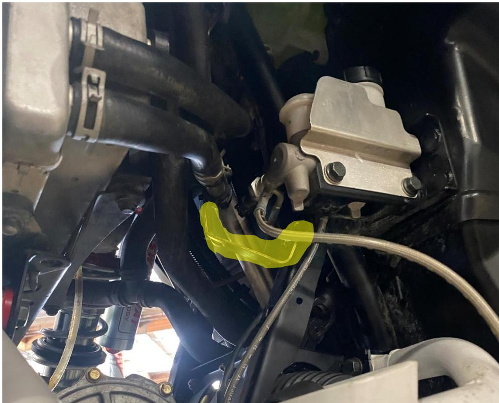
13b. With the bracket moved away from the frame, pull down the highlighted radiator hose and route beneath electric fan shroud.
