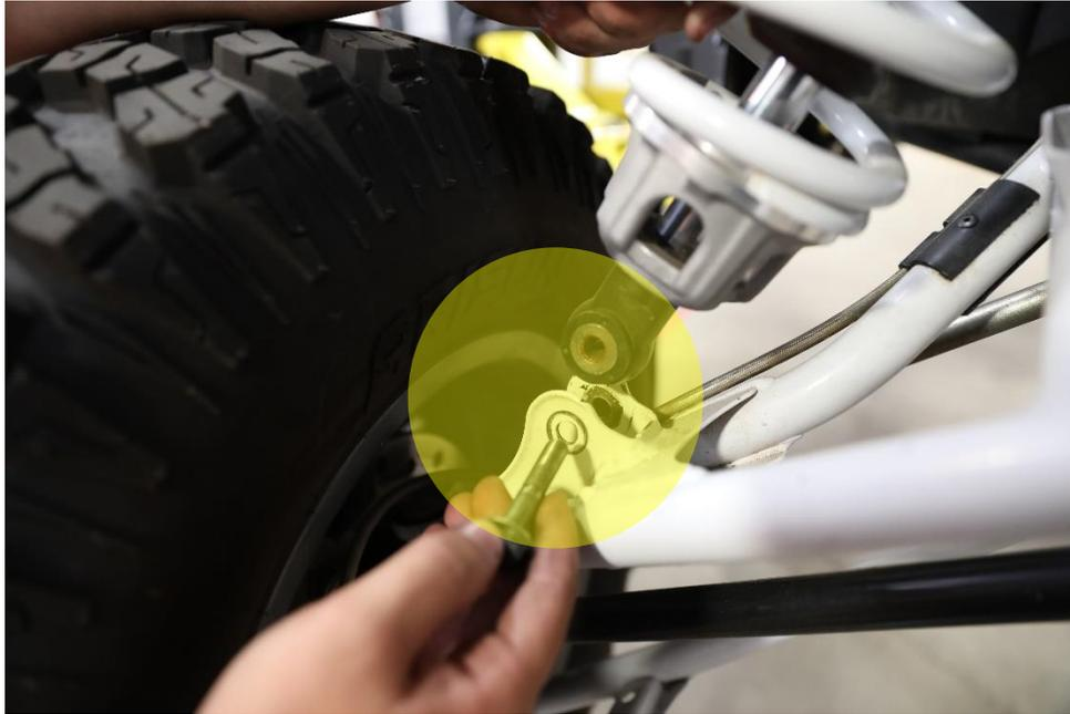
10. Remove the 15mm bolt and nut from the upper mount.
