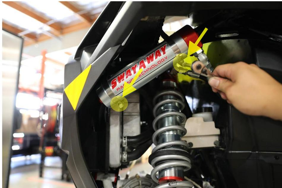
18. Double check that every bolt that was removed has been retightened. Reinstall wheels and tighten lug nuts to factory spec.
