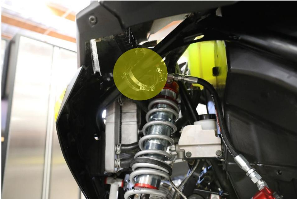
17. Put the reservoir in the location seen below and tighten the hose clamps with the rubber mounts between the reservoir and cage tubing.
