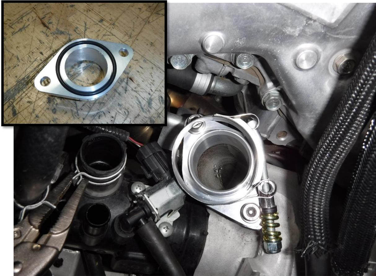
16. Install the supplied -226 O-ring into the groove on the bottom of the supplied turbo outlet flange.
