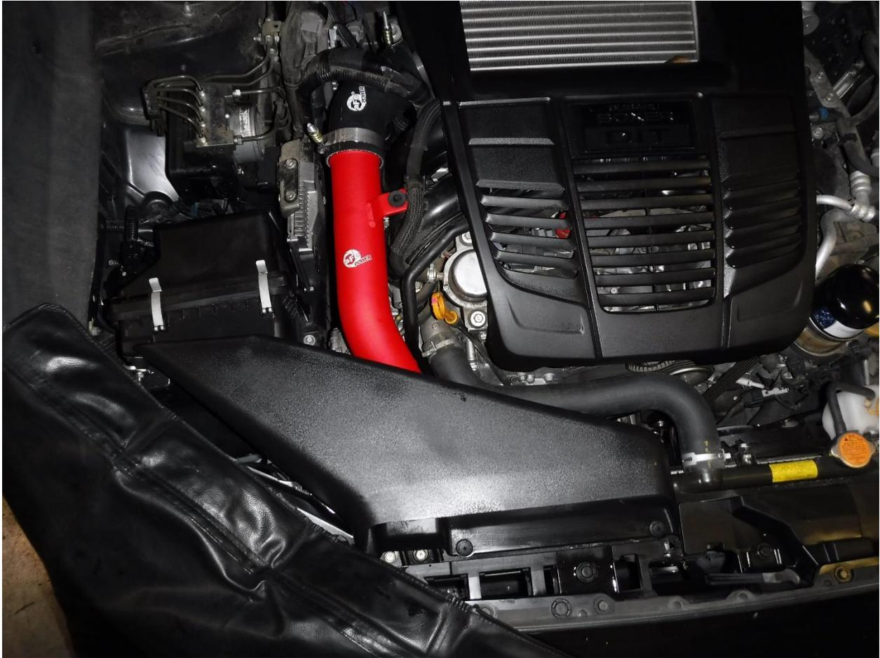
32. Reinstall the air intake scoop into the vehicle.
