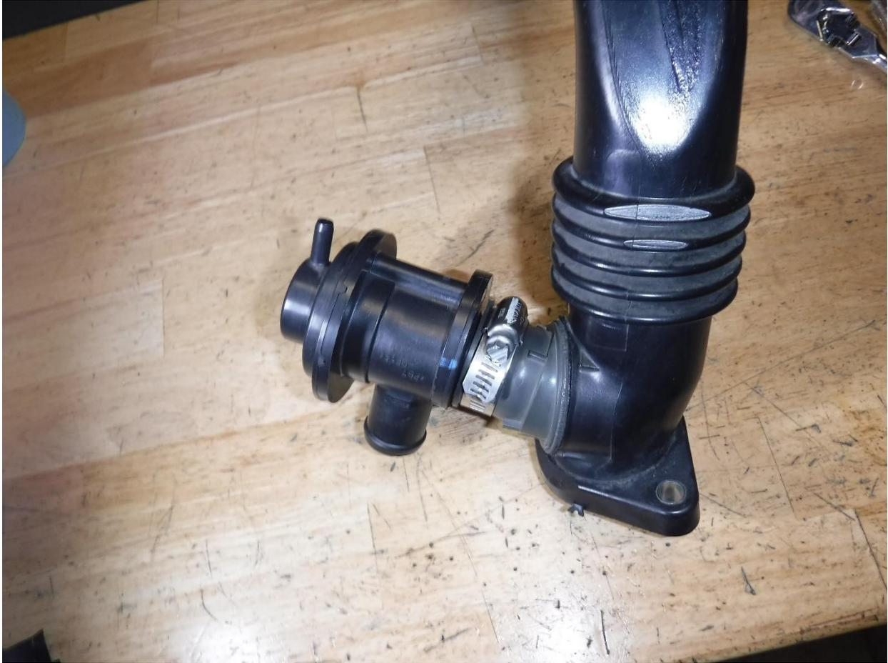
14. Loosen the clamp securing the bypass valve to the factory hot side intercooler tube.
