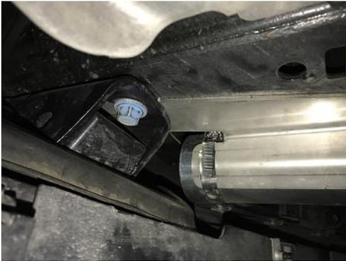
21. Place the reservoir in the bracket, position the reservoir so that the hose does not come in contact with the truck and tighten the hose clamps. Hose clamps can be slid over the outside of the reservoir and should be placed so that they are centered the openings on the bracket.
