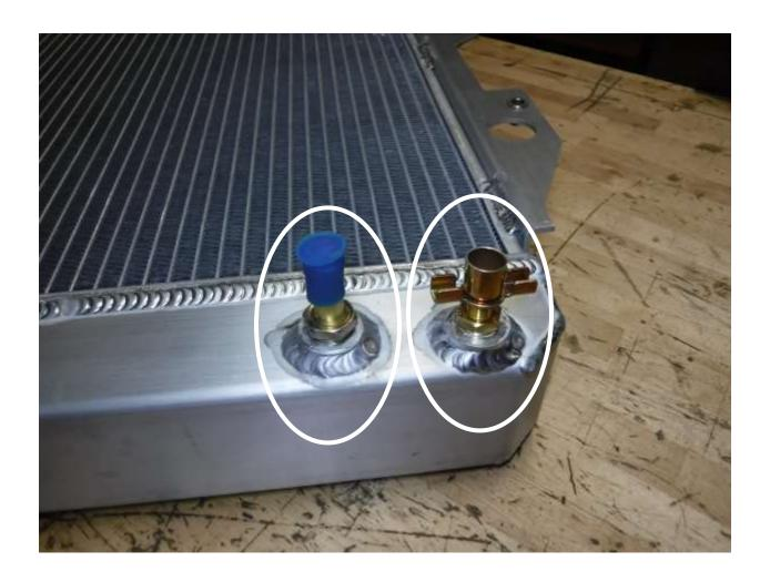
Note: Make sure to apply teflon tape to the supplied drain valve.
