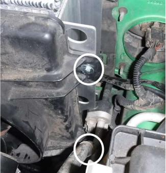
23. Tighten the fan shroud to the radiator using four (4) M6 x 1.0m x 20mm screws, four (4) M6 lock washers, and four (4) M6 fender washers. Tighten to factory specifications.
