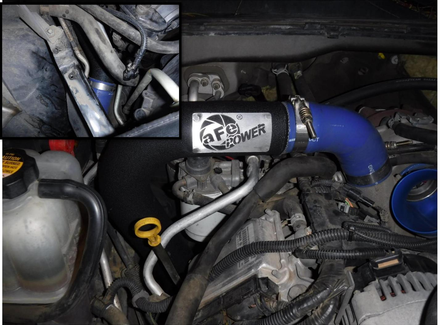
55. Reinstall the cold side intercooler tube into the vehicle, do not tighten the clamps yet.
