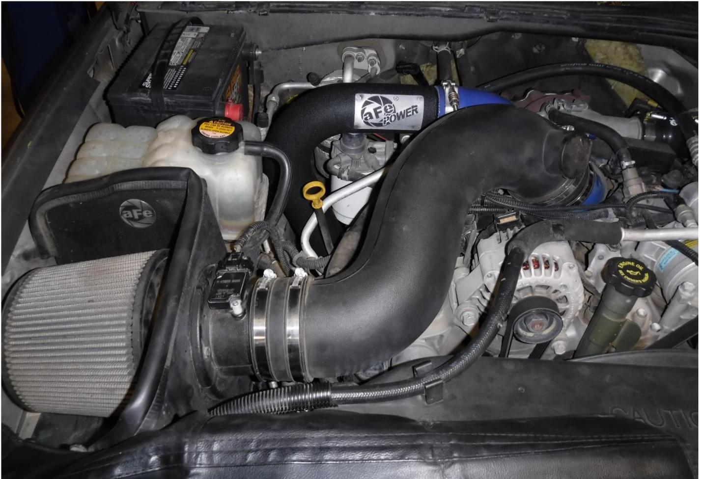
58. Reinstall the air box mounting bracket.
