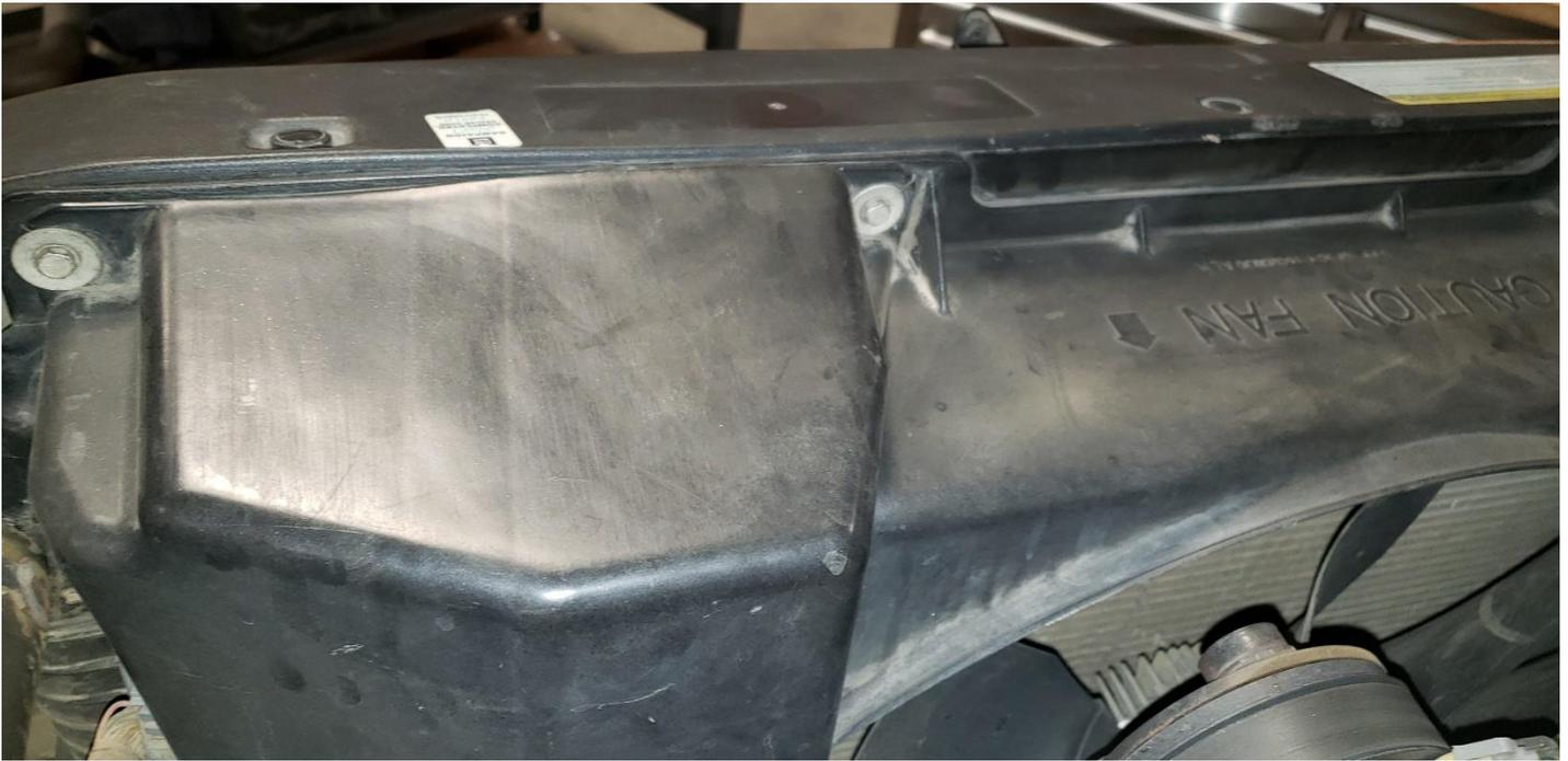
21. Remove the two (2) screws securing the computer to the fan shroud.
