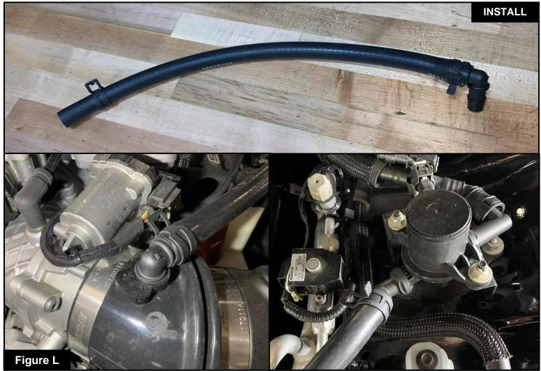
Refer to Figure L for Steps 20-21 (For SRT Hellcat Redeye and Hellcat Only)
